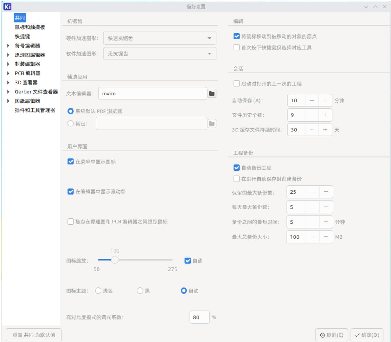
**Accelerated graphics antialiasing:** KiCad can use different methods to prevent aliasing (jagged lines) when rendering using a graphics card. Different methods may look better on different hardware, so you may want to experiment to find the one that looks best to you.
