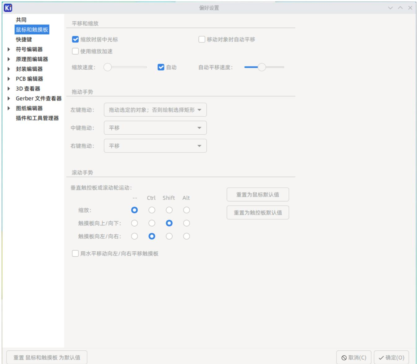
**Center and warp cursor on zoom:** When enabled, zooming using the hotkeys or mouse wheel will cause the view to be centered on the cursor location.
