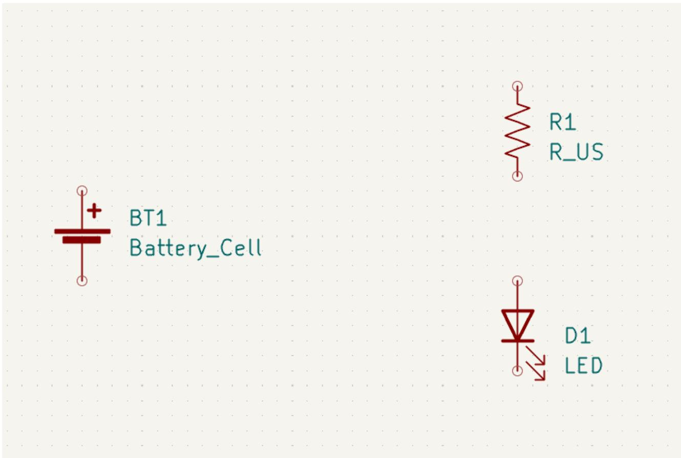
In KiCad 8.0, objects are selected by clicking on them while the selection tool is active. The selection tool is the default tool when no other tool is active, so you can enter the selection tool by quitting any active tool (`Esc`) or by clicking the
