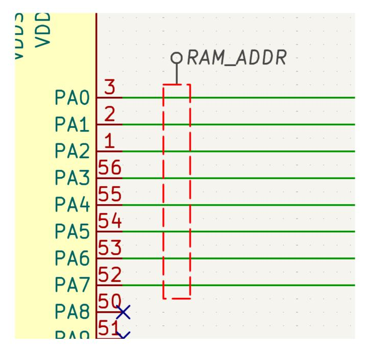
You can show or hide directive labels in the schematic using the **View**  $\rightarrow$  **Show Directive Labels** option.
