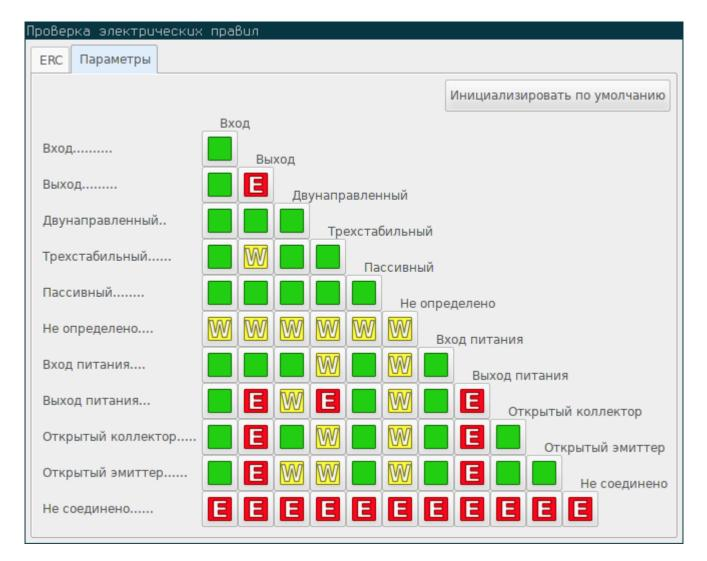
Rules can be changed by clicking on the desired square of the matrix, causing it to cycle through the choices: allowed, warning, error.
