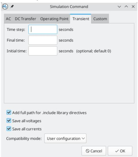
Calculates the time-varying behavior of the circuit.
