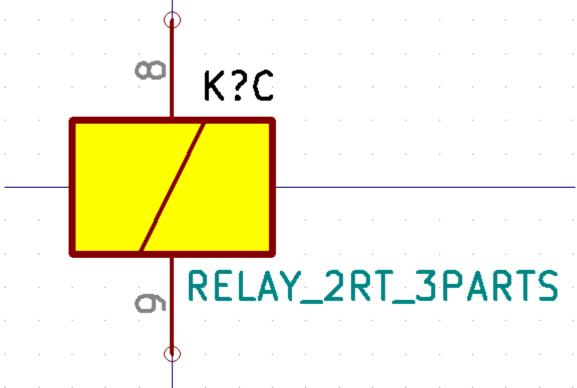
Unit A does not have the same symbol and pin layout as Units B and C, so the units are not interchangeable.
