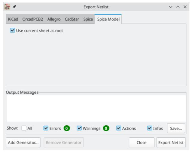
KiCad can also export a netlist of the schematic as a Spice subcircuit model, which can be included in a separate Spice simulation. Any hierarchical labels in the schematic are used as pins for the subcircuit model. Each pin in the model is annotated with a comment describing the pin's electrical direction:
