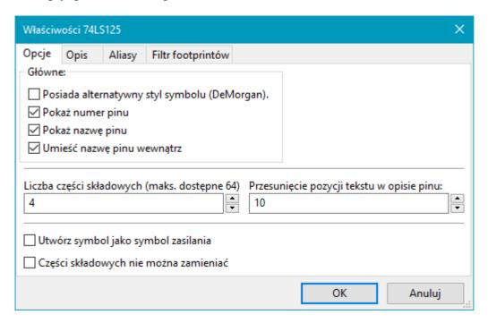
It is important to set the **number of units** and check **all units are interchangeable** and **has alternate body style**, as applicable, because these settings affect how pins and graphics are added to each symbol unit.
