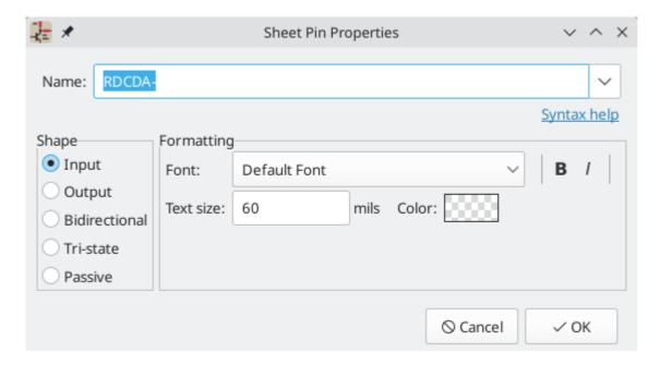
The sheet pin's **name** can be edited in the textbox or by selecting from the dropdown list of hierarchical labels in the subsheet. A sheet pin's name has to match the corresponding hierarchical label in the subsheet, so if a pin name is changed the label must change as well.
