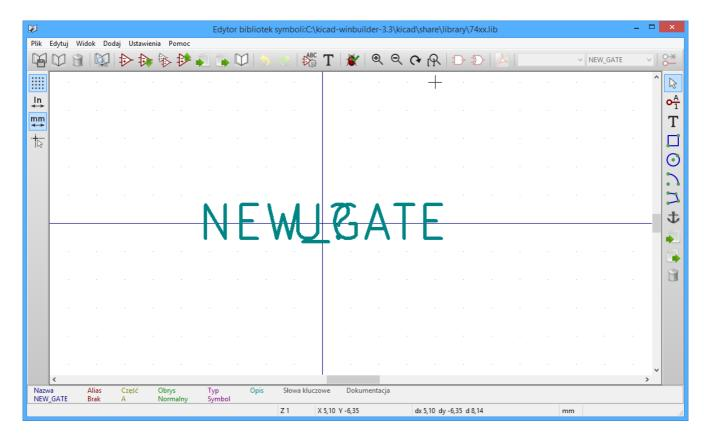
The blue cross in the center is the symbol anchor, which specifies the symbol origin i.e. the coordinates (0, 0). The anchor can be repositioned by selecting the \* button and clicking on the new desired anchor position.
