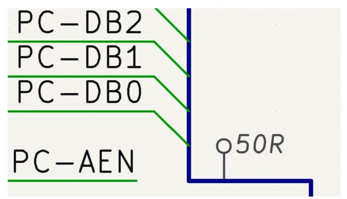
Directive labels are added with the **A** button in the right toolbar. They behave like labels, except that they cannot be used to name a net. The attached net is assigned a net class according to the value of the directive's Net Class field. The Net Class field presents a dropdown list of all the net classes in the design.
