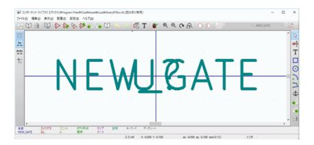
The blue cross in the center is the symbol anchor, which specifies the symbol origin i.e. the coordinates (0, 0). The anchor can be repositioned by selecting the specifies the symbol and clicking on the new desired anchor position.
