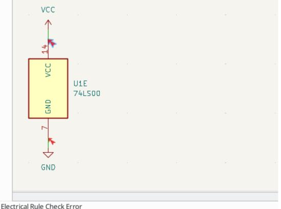
Input Power pin not driven by any Output Power pins
