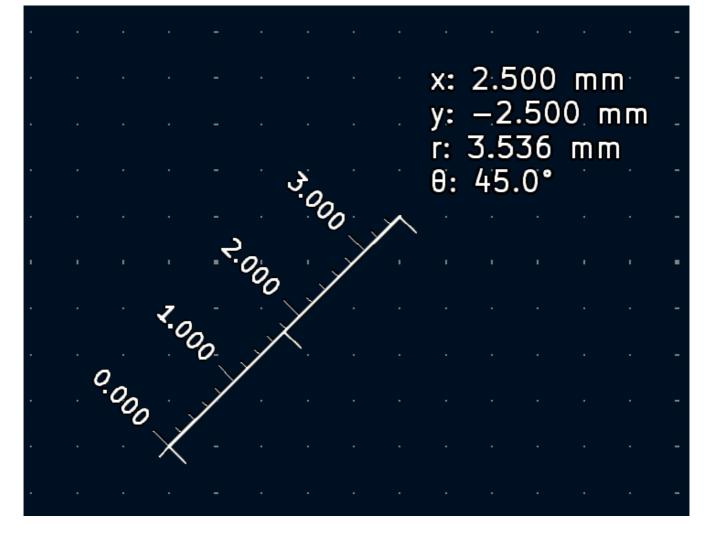
The tool displays the total (radial) distance between the points, the distance in X and Y directions, and the measured angle from horizontal. In other words, both the Cartesian and radial (polar) distances are displayed.
