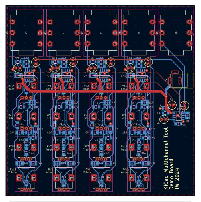
Using the multichannel layout feature first requires you to designate which portions of the schematic represent the repeated parts of the circuit. You can either use hierarchical sheets, with a repeated hierarchical sheet for each channel, or component classes with a unique component class assigned to the symbols in each channel. Each channel will exactly correspond to the symbols (and their associated connections) in a single sheet or component class.
