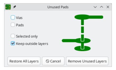
The **Remove Unused Layers** button removes all unused annular rings from pads and vias that meet the selected filter settings. The **Restore All Layers** button restores all annular rings to the pads and vias that meet the selected filter settings.
