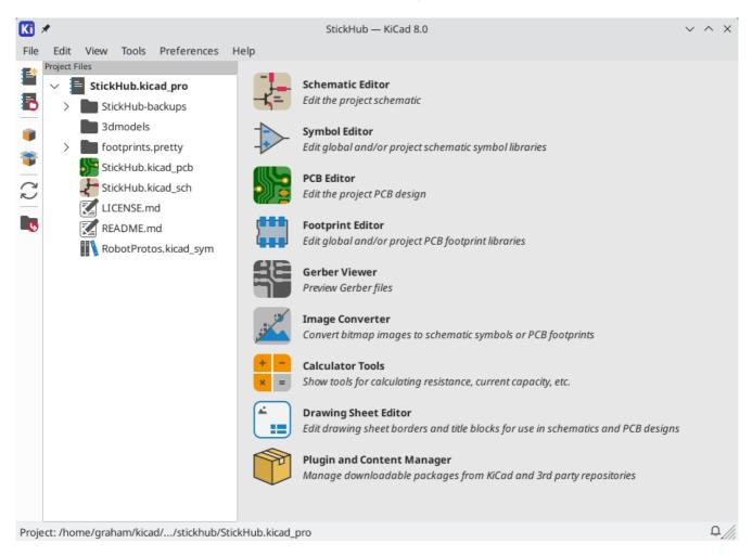
The KiCad project manager window is composed of a tree view on the left showing the files associated with the open project, and a launcher on the right containing shortcuts to the various editors and tools.
