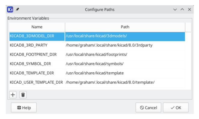
Paths set in the Configure Paths dialog are internal to KiCad and are not visible as environment variables outside of KiCad. They are stored in KiCad's user configuration files.
