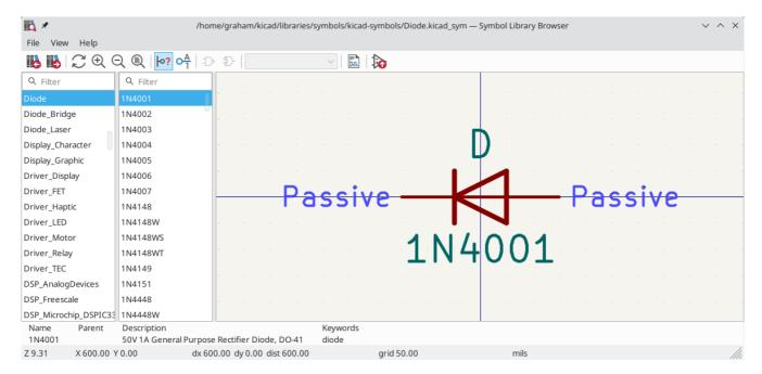
Double clicking the name of a symbol or using the houton adds the symbol to the schematic.
