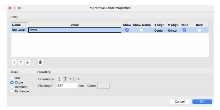
In addition to the associated net class, you can edit the directive's **shape** (dot, circle, diamond, or rectangle), **orientation**, **pin length**, and **color** in the directive's properties.
