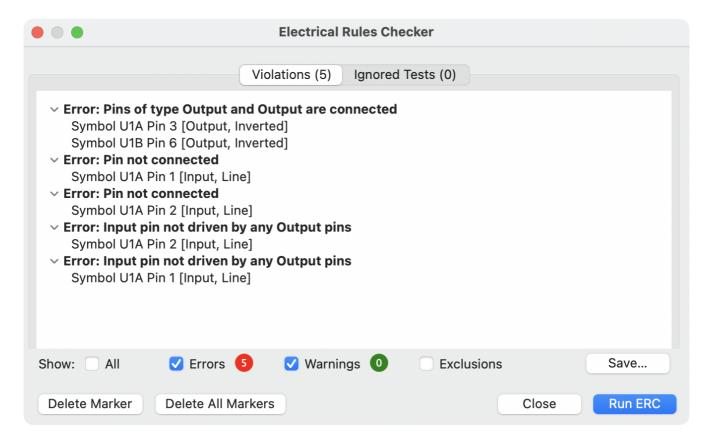
Any warnings or errors are reported in the **Violations** tab, and markers for each violation are placed in the schematic so that they point to the relevant part of the schematic. Warnings are indicated by yellow arrows, and errors have red arrows. Excluded violations are shown as green arrows. A list of the ignored tests are shown in the **Ignored Tests** tab. A report file in plain text format can be created after running DRC using the **Save...** button.
