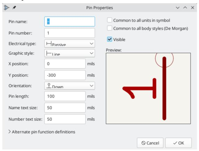
The pin properties dialog allows you to edit all of the characteristics of a pin. This dialog pops up automatically when you create a pin or when double-clicking on an existing pin. This dialog allows you to modify:
