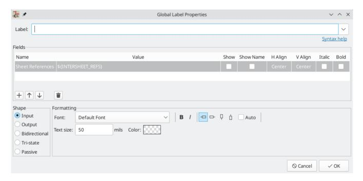
The **Label** field sets the label's text, which determines the net that the label assigns to its attached wire. Label text supports markup for overbars, subscripts, etc., as well as variable substitution. Use the **Syntax help** link in the dialog for a summary.
