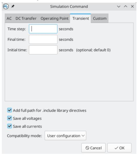
Calculates the time-varying behavior of the circuit.
