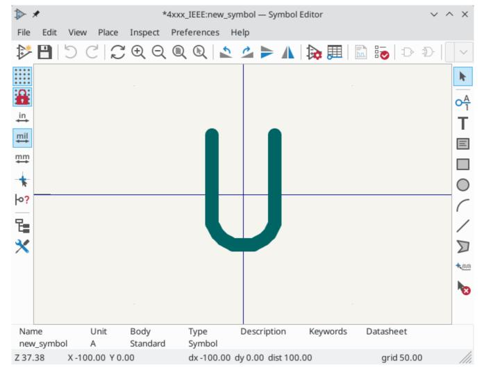
The blue cross in the center is the symbol anchor, which specifies the symbol origin i.e. the coordinates (0, 0). The anchor can be repositioned by selecting the hour and clicking on the new desired anchor position.
