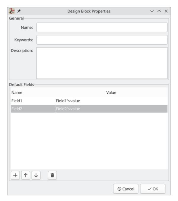
This brings up the Design Block Properties dialog, where you can edit the properties of the new design block.
