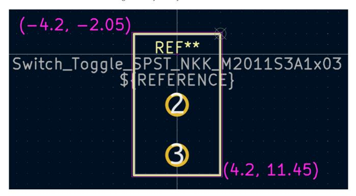
After completing the outlines, position the text as shown below. The footprint is complete.
