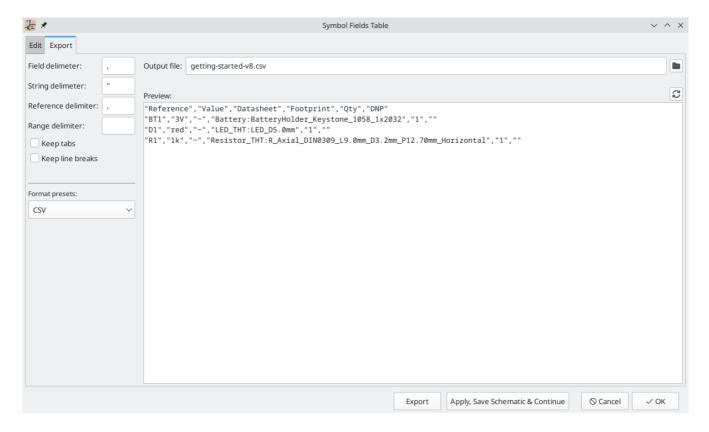
KiCad 8.0 has a GUI for BOM export. You can configure which symbol metadata will be exported, and how the symbols are grouped, in the **Edit** tab, and configure the output format in the **Export** tab.
