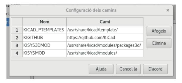
Paths set in the Configure Paths dialog are internal to KiCad and are not visible as environment variables outside of KiCad. They are stored in KiCad's user configuration files.
