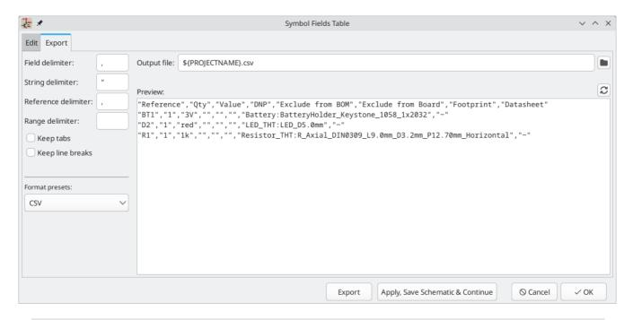
KiCad has a GUI for BOM export. You can configure which symbol metadata will be exported, and how the symbols are grouped, in the **Edit** tab, and configure the output format in the **Export** tab.
