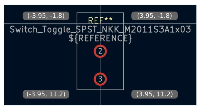
Next, switch to the F.Silkscreen layer. We want the silkscreen outline to be just outside of the part outline, so the silkscreen lines will be drawn 0.11 mm to the outside of the lines on the fabrication layer (0.11 mm is half of the 0.10 mm fab line width, plus half of the 0.12 mm silkscreen line width). The exact coordinates are shown in the screenshot below, and helpful grid settings are:
