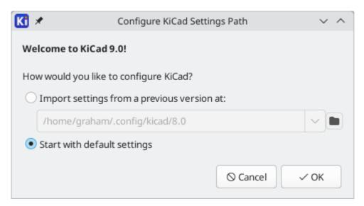
If a previous version of KiCad is detected, you will have the option to import the settings from that version. The location of the previous configuration files is detected automatically, but you may override it to choose another location if desired.
