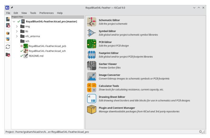
The KiCad project manager window is composed of a tree view on the left showing the files associated with the open project, and a launcher on the right containing shortcuts to the various editors and tools.
