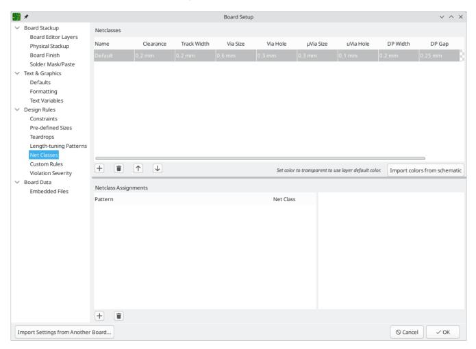
Track width and spacing can be managed manually by the designer during layout, but net classes are recommended because they provide an automatic way to manage and check design rules.
