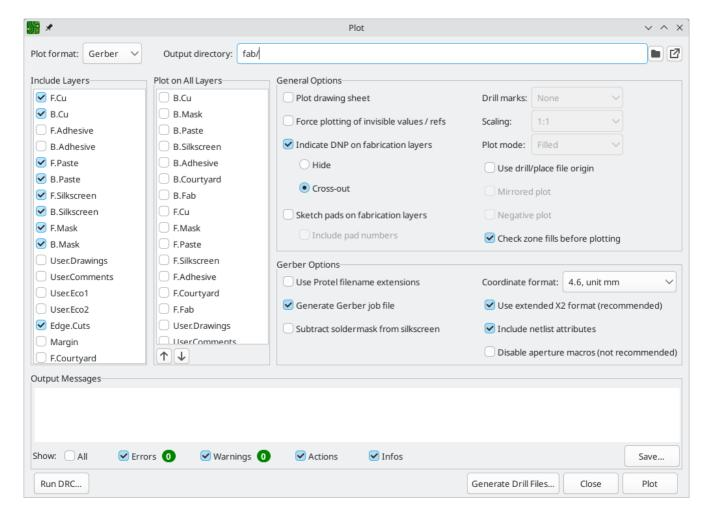
Click **Plot** to generate the Gerber files. Also click **Generate Drill Files...** and then **Generate Drill File** to create files specifying the location of all holes that will be drilled in the board. Finally, close the Plot dialog. The design is finished.
