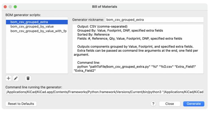
Additional scripts can be added to the list of BOM generator scripts by clicking the + button. Scripts can be removed by clicking the 👕 button. The 🖋 button opens the selected script in a text editor.
