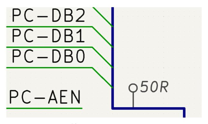
Directive labels are added with the **A** button in the right toolbar. They behave like labels, except that they cannot be used to name a net. The attached net is assigned a net class according to the value of the directive's Net Class field. The Net Class field presents a dropdown list of all the net classes that have been specified in Schematic Setup or Board Setup.
