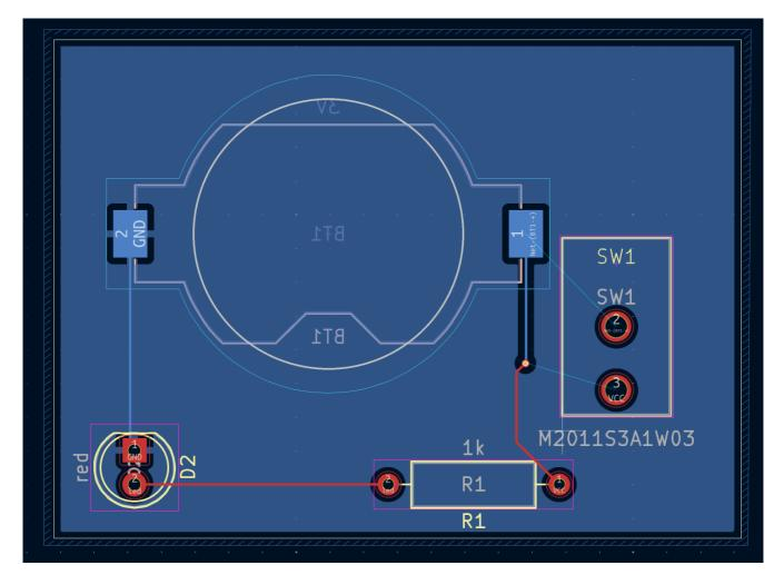
The ratsnest shows the new connections that need to be routed. Additionally, the connection between the battery and the resistor needs to be deleted.
