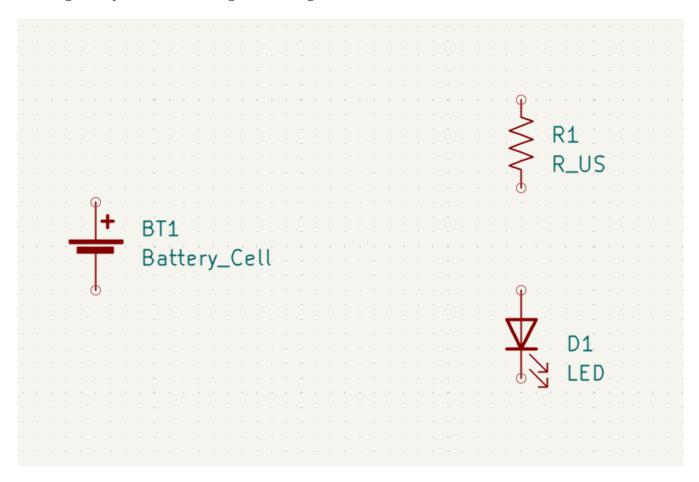
In KiCad, objects are selected by clicking on them while the selection tool is active. The selection tool is the default tool when no other tool is active, so you can enter the selection tool by quitting any active tool (Esc ) or by clicking the button in the right toolbar.
