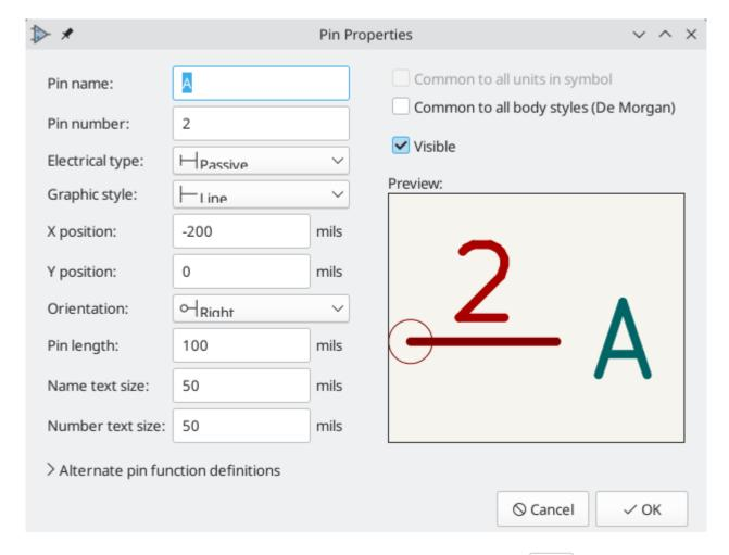
Add a second pin, but this time don't use the **Add a pin** tool. Instead, press Insert. A new pin numbered 3 is added to the symbol, just below pin 2.
