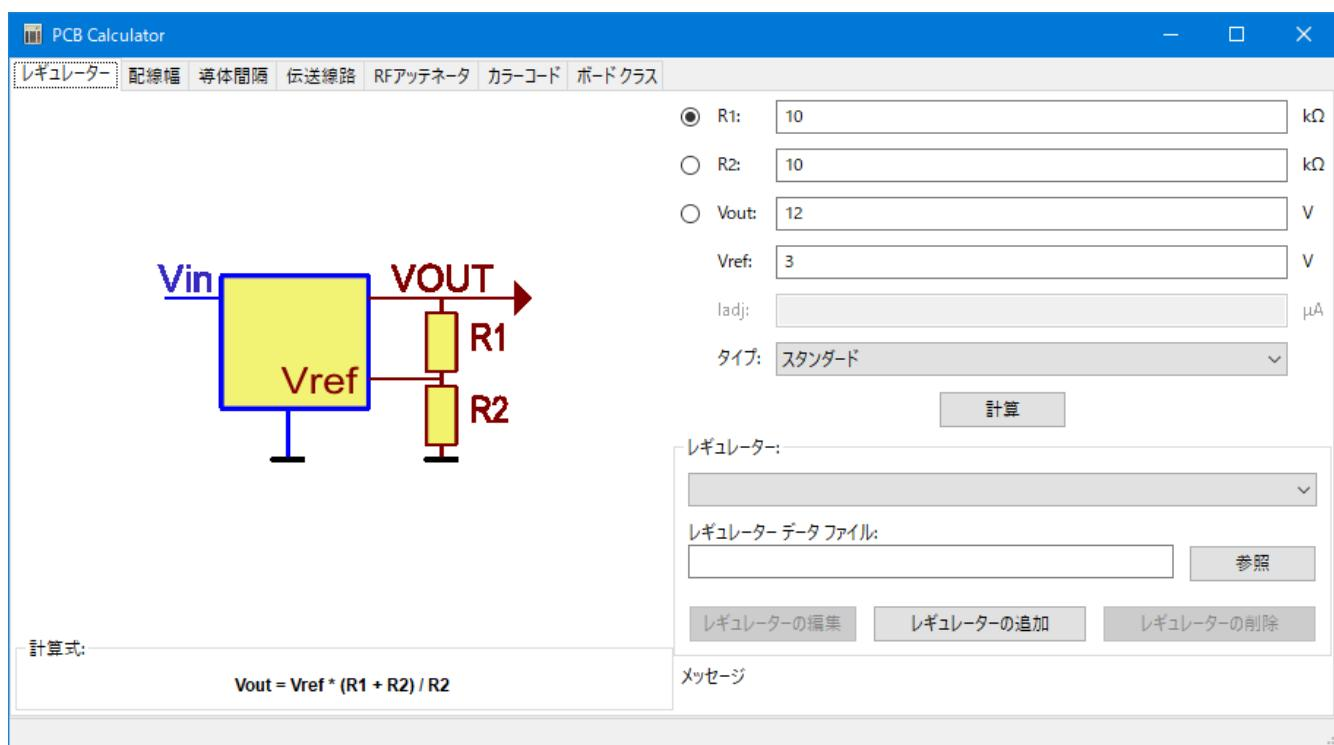
For the *Standard Type*, the output voltage  $V_{out}$  as a function of the reference voltage  $V_{ref}$  and resistors  $R_1$  and  $R_2$  is given by:
