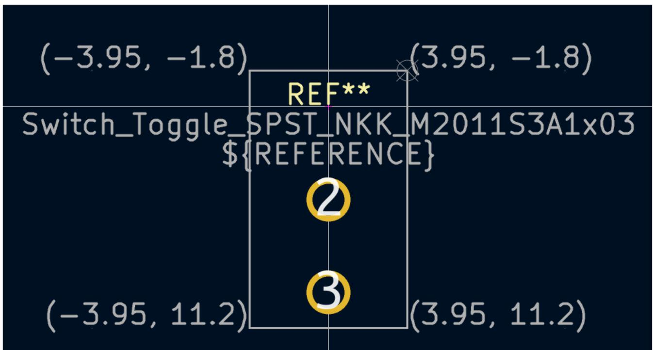
Next, switch to the **F.Silkscreen** layer. The silkscreen outline should be just outside of the part outline, so the silkscreen lines are moved outwards from the fabrication drawing by 0.11 mm (half of 0.10 mm fab line
