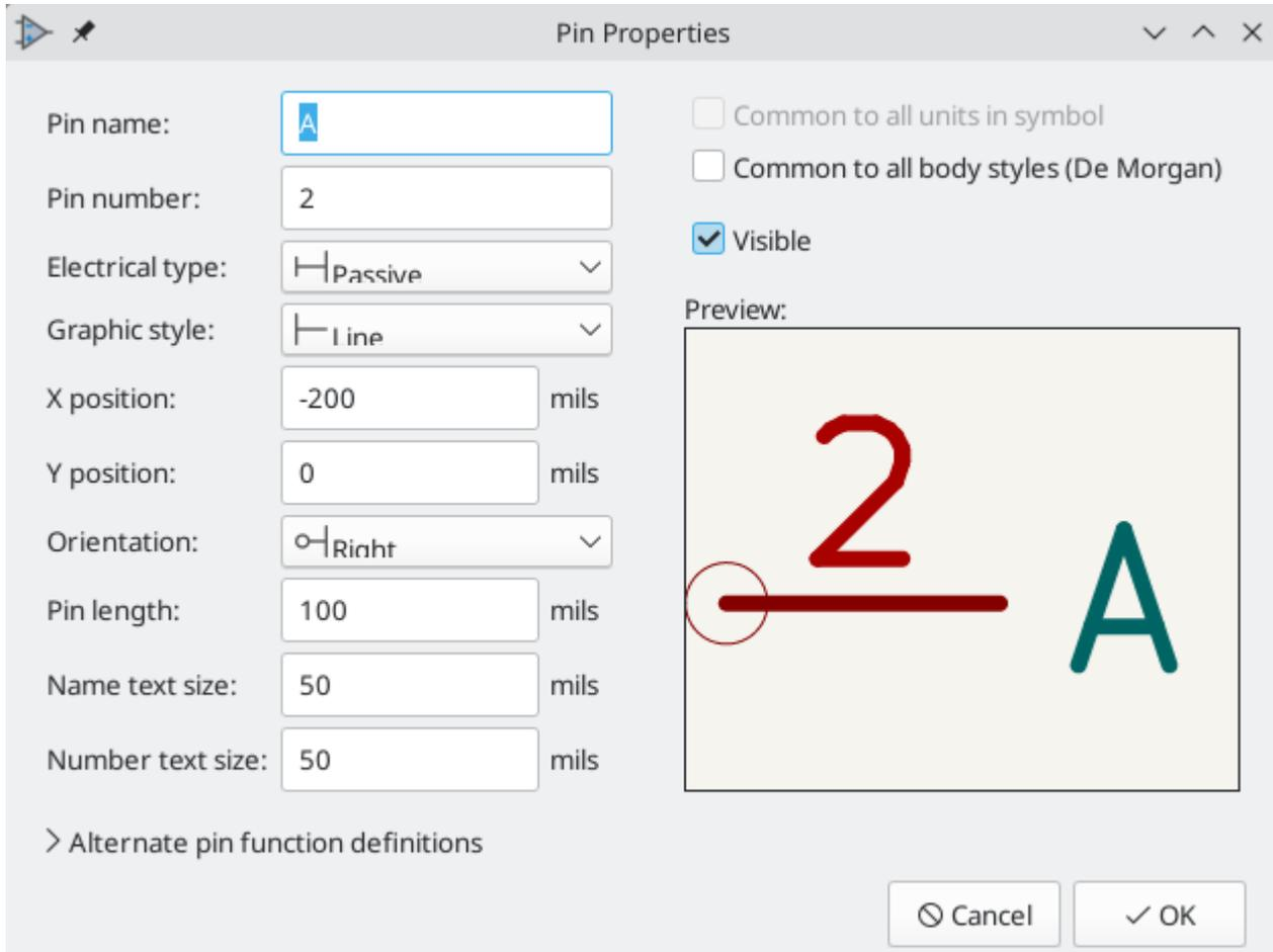
Add a second pin, but this time don't use the **Add a pin** tool. Instead, press **Insert**. A new pin numbered 3 is added to the symbol, just below pin 2.
