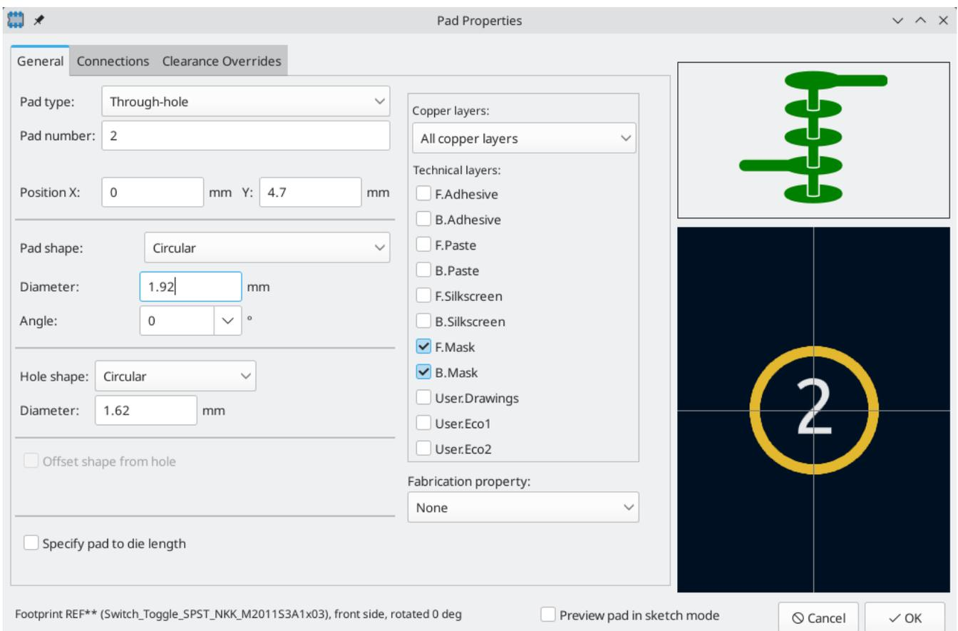
Now use the **Add a pad** tool again to place the other pad at (0, 9.4 mm). Notice that the pad number is automatically incremented and the properties including pad size and hole size are copied from the previous pad.
