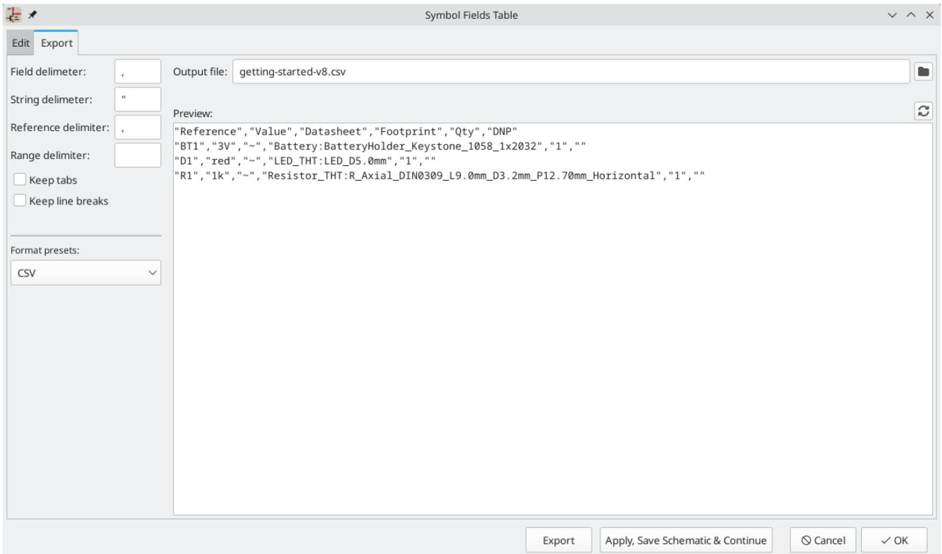
KiCad 8.0 has a GUI for BOM export. You can configure which symbol metadata will be exported, and how the symbols are grouped, in the **Edit** tab, and configure the output format in the **Export** tab.
