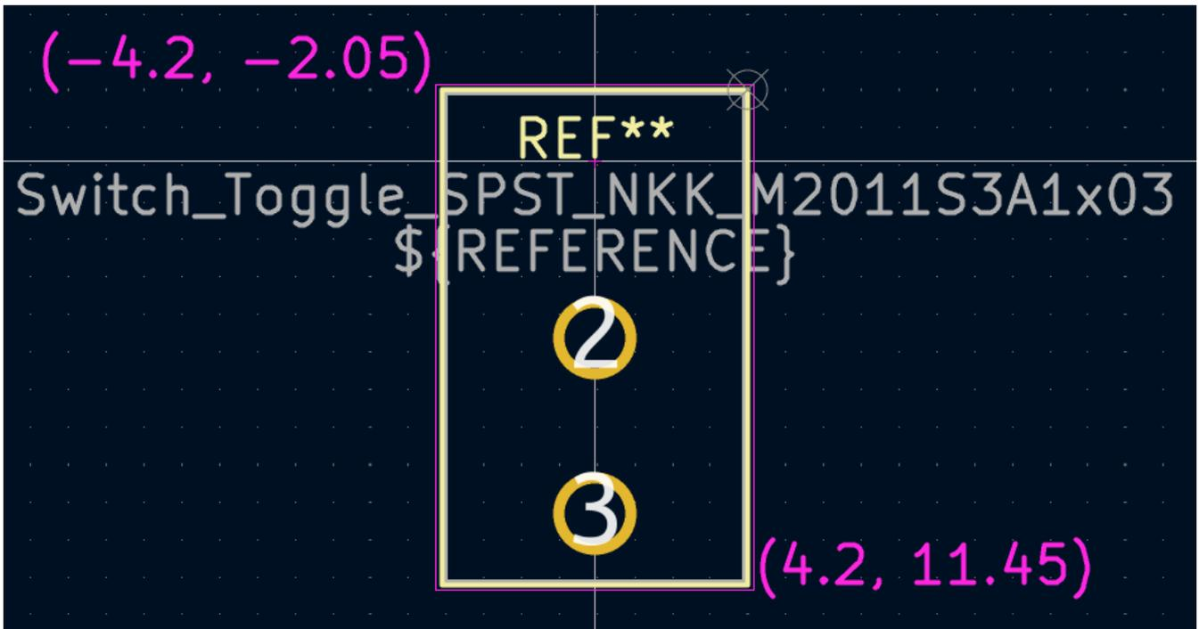
After completing the outlines, position the text as shown below. The footprint is complete.
