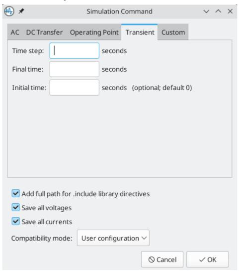
Calculates the time-varying behavior of the circuit.
