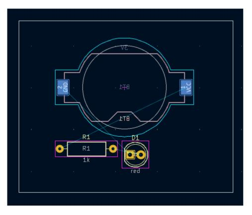
All PCB layers are viewed from front side of the board. Footprints on the bottom of the board are therefore upside down and appear mirrored.
