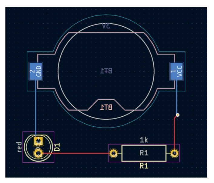
At this point, all connections are routed. This can be confirmed by looking at the status screen in the bottom left of the window, where the number of unrouted nets is given as 0.
