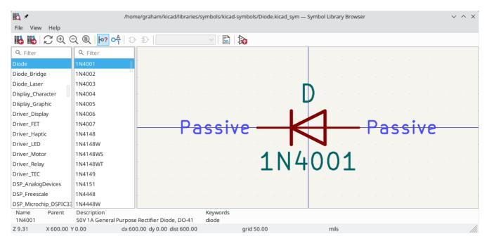
Double clicking the name of a symbol or using the 🍌 button adds the symbol to the schematic.
