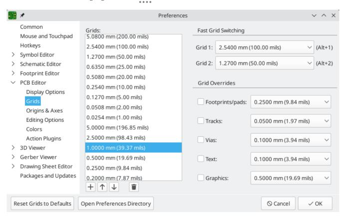
In this dialog you can select an active grid from the list of grids, reorder the list of grids, and add or remove grids. Grids defined in this dialog can have unequal X and Y spacing as well as an optional name.
