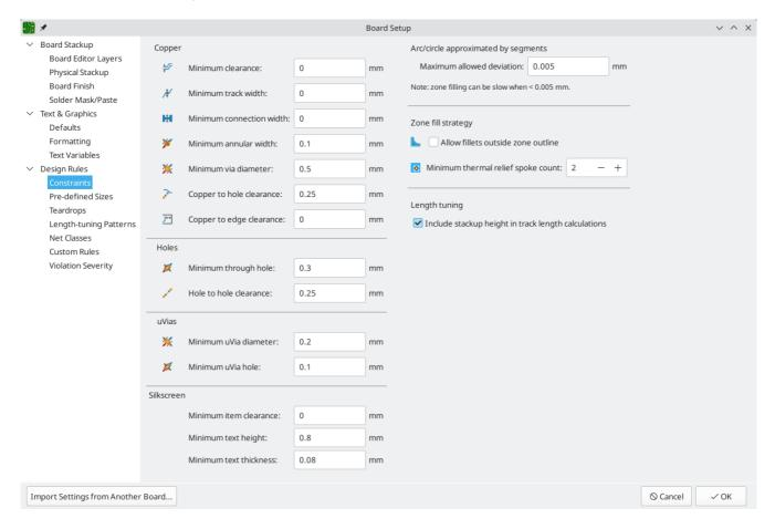
In addition to setting minimum clearances, a number of features can be configured here:
