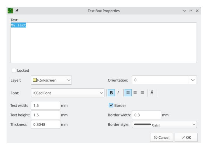
**Locked** controls whether or not the text object is locked. Locked objects may not be manipulated or moved, and cannot be selected unless the **Locked Items** option is enabled in the Selection Filter panel.
