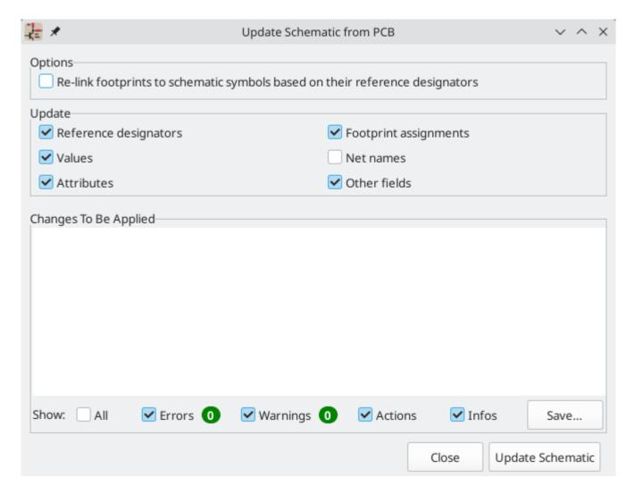
The tool syncs changes in reference designators, values, footprint assignments, and net names from the board to the schematic. Each type of change can be individually enabled or disabled.
