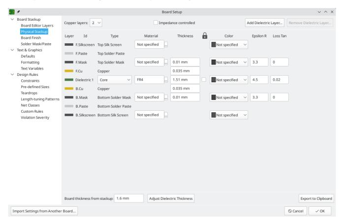
Set the number of copper layers in the upper left corner and then enter the physical parameters of the stackup if desired. These parameters may be left at their default values, but note that the board thickness value will be used when exporting a 3D model of the board, and layer thicknesses will be included in net length calculations for any nets that include vias. If you plan to use these features, it is a good idea to ensure that the stackup thickness is correct.
