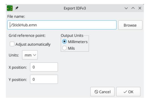
**Grid reference point:** Choose where the exported model's reference point should be. If the **Adjust automatically** option is selected, KiCad will set the reference point to the centroid of the PCB. Otherwise, the reference point is set relative to the display origin.
