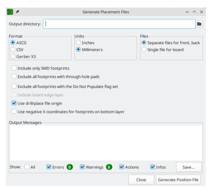
**Format:** Choose between generating a plain text (ASCII), comma-separated text (CSV), or Gerber X3 placement file format.
