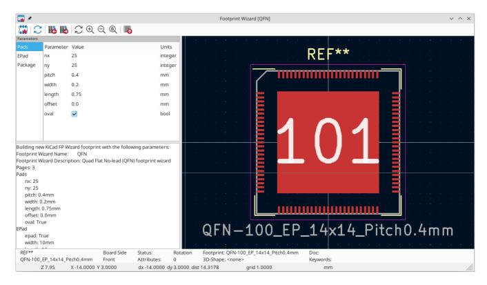
In the window that appears, fill out the parameters as appropriate. When the parameters are correctly filled out, press the button to transfer the generated footprint back into the footprint editor. Then you can make additional manual modifications and save the footprint as normal.
