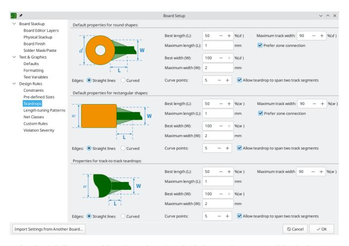
Rather than in bulk, you can add or edit teardrops for individual vias in the properties dialog for that via, or for individual pads in the **Connections** tab of the pad's properties dialog. The settings in the properties dialogs are the same as in the Edit Teardrops dialog. You can also edit teardrops for individual pads and vias with the Properties Manager.
