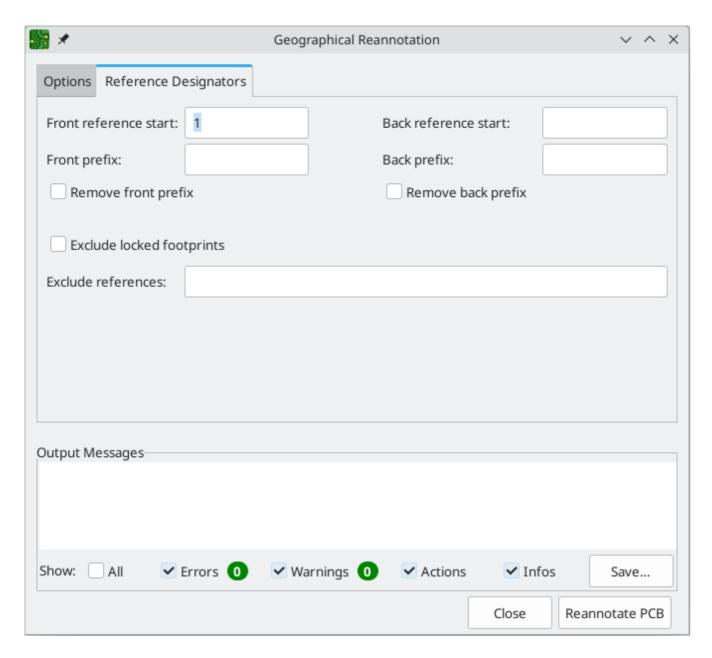
The **Reference Designators** tab contains options for how to allocate new reference designators. There are separate settings for footprints on the front and back of the board.
