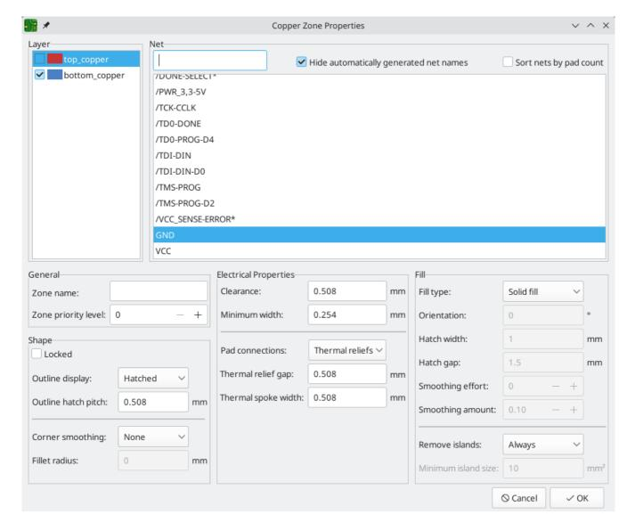
**Layer:** A single zone object can create filled copper on one or more copper layers. Check the box next to each copper layer that this zone outline should fill on. The copper on each layer will be filled independently, but all layers will share the same net.
