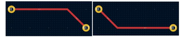
KiCad's router attempts to pick the best posture automatically based on a number of factors. In general, the router will attempt to minimize the number of corners in a route, and will avoid "bad" corners such as acute angles whenever possible. When routing from or to a pad, KiCad will choose the posture that lines up the route with the longest edge of the pad.
