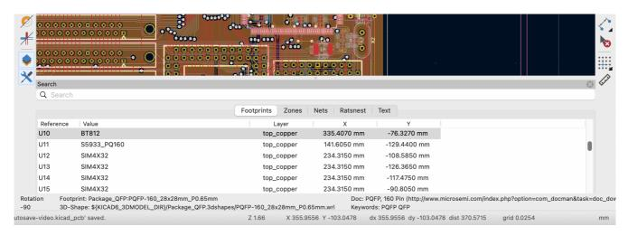
Items are filtered based on their properties: footprints are filtered by their reference designator and value, zones by the zone name, net and ratsnest items by the net name, and text (text, textboxes, and dimensions) by the text content. You can sort the filtered results in ascending or descending order of the value in a particular column by clicking on that column header.
