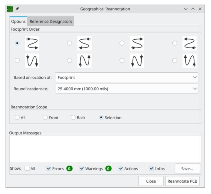
The **Options** tab contains settings for how footprint locations affect reannotation. The arrow diagrams indicate which geographical ordering to use when reannotating. You can reannotate from left-to-right, right-to-left, top-to-bottom, or bottom-to-top, and you can select whether to use a column-major order (go through all footprints in the same column before moving to the next column) or row-major order (go through all footprints in the same row before moving to the next row).
