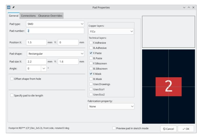
**Pad type:** this setting controls which features are enabled for the pad:
