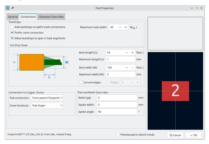
The Teardrops section contains settings controlling teardrop connections between tracks and the pad, if teardrops are used. Teardrop settings are explained in the teardrop documentation.
