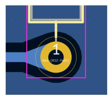
You can add teardrops to your design in bulk using the **Edit**  $\rightarrow$  **Edit Teardrops...** dialog. This dialog has controls for filtering which objects are affected and settings for configuring the shape of the new teardrops. It also lets you edit or remove existing teardrops.
