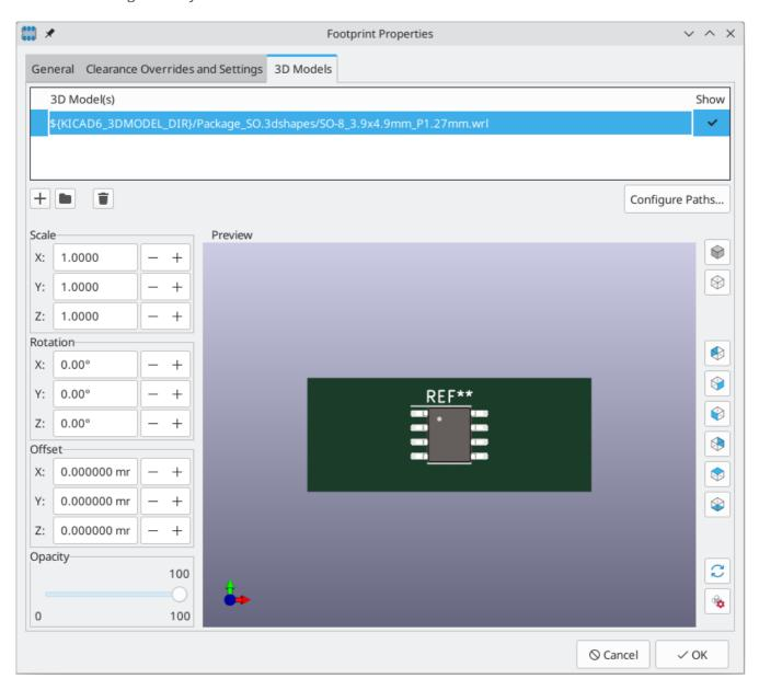
The main part of the window is a 3D preview of the footprint and any attached models. The buttons to the right of the preview let you enable or disable an orthographic projection (), show or hide the PCB model (), align the view to one of the six face-aligned perspectives (), and refresh the view (). The bottom button () lets you set the thickness of the PCB in the preview.
