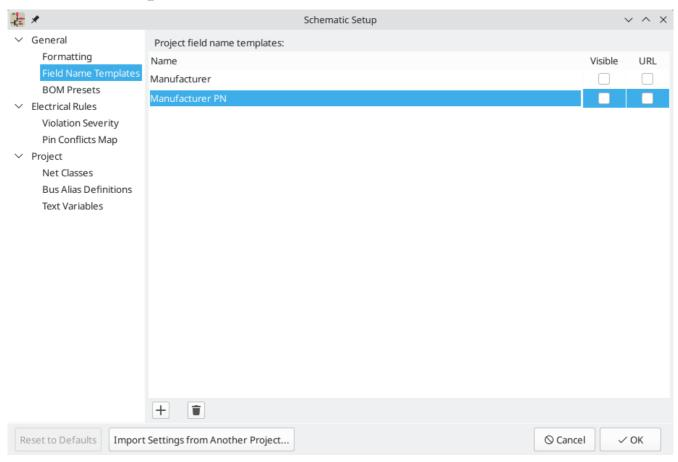
Field name templates are empty symbol fields that are automatically added to all symbols in the schematic. These can be useful when every symbol in the schematic needs additional fields beyond the fields that are defined in the library symbols, for example a field for the manufacturer's part number.
