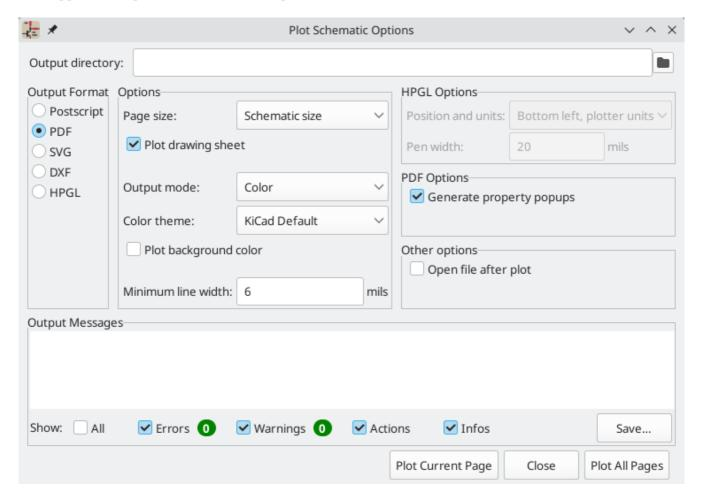
The **Output Messages** pane displays messages about the generated files. Different kinds of messages can be shown or hidden using the checkboxes, and the messages can be saved to a file using the **Save...** button.
