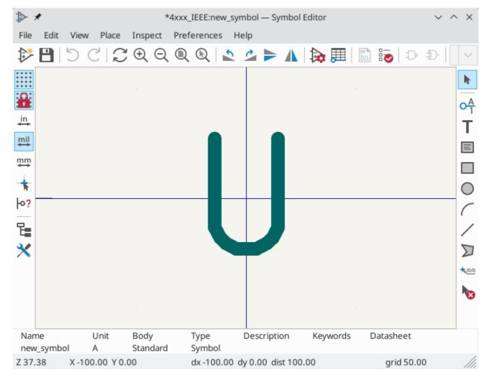
The blue cross in the center is the symbol anchor, which specifies the symbol origin i.e. the coordinates (0, 0). The anchor can be repositioned by selecting the \* button and clicking on the new desired anchor position.
