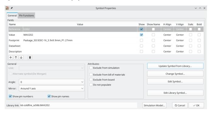
You can only use the properties dialog to edit one item at a time. To edit multiple items, use the properties manager, described below. There are also other tools that can be used to edit specific types of objects in bulk, such as the Edit Text and Graphics tool for editing text, labels, and graphic shapes, or the Symbol Fields Table for editing symbol fields in bulk.
