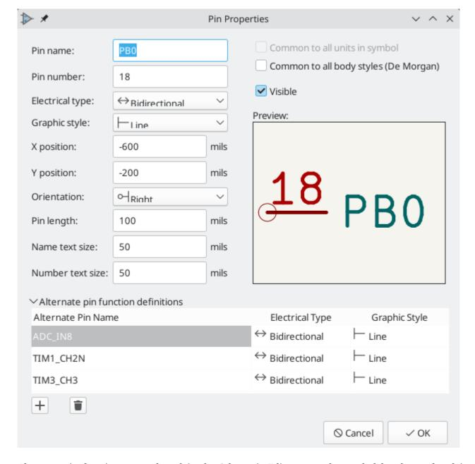
Alternate pin functions are selected in the Schematic Editor once the symbol has been placed in the schematic. The alternate pin is assigned in the **Pin Functions** tab of the Symbol Properties dialog. Alternate definitions are selectable in the dropdown in the Alternate Assignment column. You can also select an alternate pin by right-clicking the pin and selecting a new function from the **Pin Function** menu.
