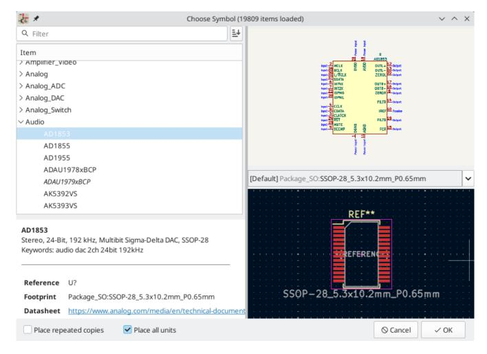
Symbols can have footprint filters that specify which footprints are appropriate to use with that symbol. If footprint filters are defined for the selected symbol, all footprints that match the footprint filters will appear as options in the footprint dropdown. The selected footprint will be displayed in the preview canvas and will be assigned to the symbol when the symbol is added to the schematic.
