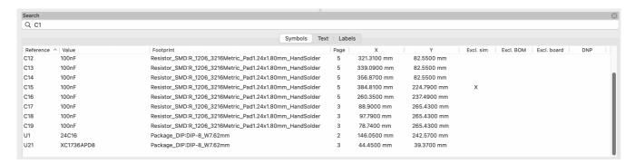
Items are filtered based on their properties: symbols are filtered by all non-hidden fields, text (text and textboxes) by the text content, and labels by their netname. You can sort the filtered results in ascending or descending order of the value in a particular column by clicking on that column header.
