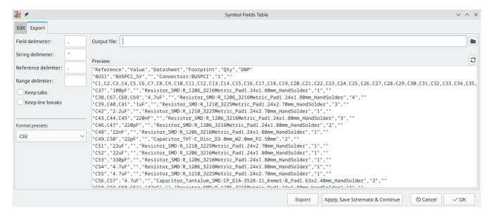
At the top you can specify the output file. Pressing the **Export** button will write the BOM to this file path. This path can contain text variables.
