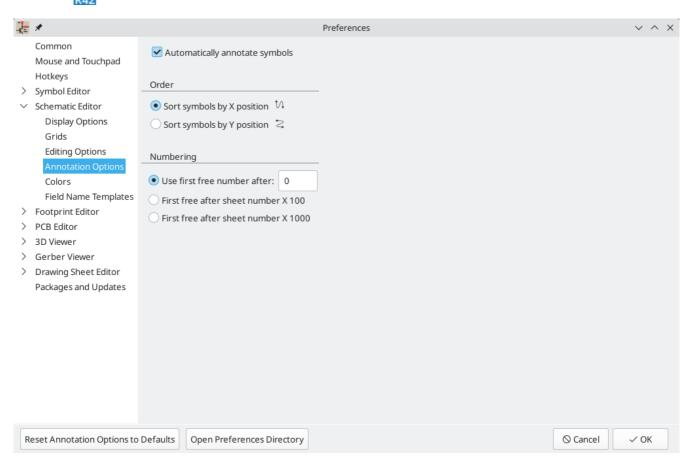
When multiple symbols are added simultaneously, they are annotated according to the **Order** setting, sorted by either X or Y position.
