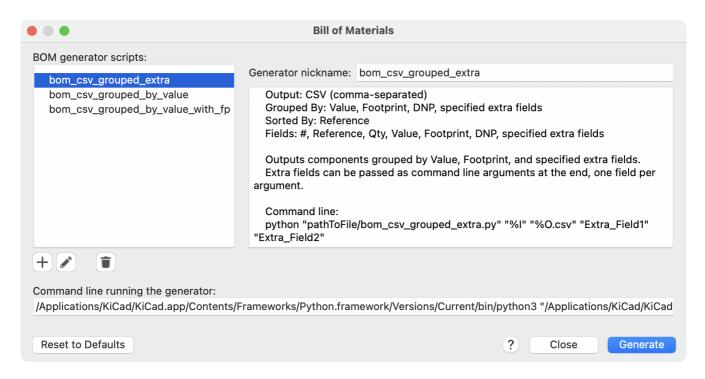
Additional scripts can be added to the list of BOM generator scripts by clicking the + button. Scripts can be removed by clicking the = button. The  $\nearrow$  button opens the selected script in a text editor.
