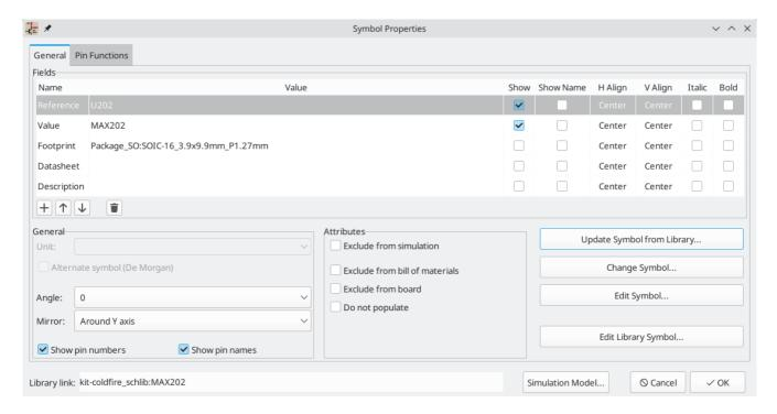
The Symbol Properties window displays all the fields of a symbol in a table. New fields can be added, and existing fields can be deleted, edited, reordered, moved, or resized. Fields can be arbitrarily named, but names beginning with ki\_, e.g. ki\_description, are reserved by KiCad and should not be used for user fields.
