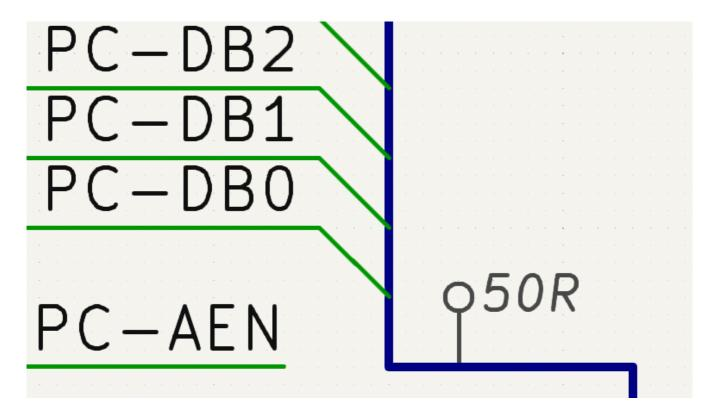
Net class directives are added with the QA button in the right toolbar. They behave like labels, except that they cannot be used to name a net. The attached net is assigned a netclass according to the value of the directive's Net Class field. The Net Class field presents a dropdown list of all the net classes in the design.
