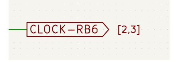
A Sheet References field with value \${INTERSHEET\_REFS} is automatically added to global labels, and is used to control the appearance of inter-sheet references for that label. The \${INTERSHEET\_REFS} text
