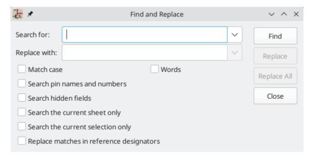
If the **Replace matches in reference designators** option is checked, reference designators will be modified if they contain matching text. Otherwise reference designators will not be affected.
