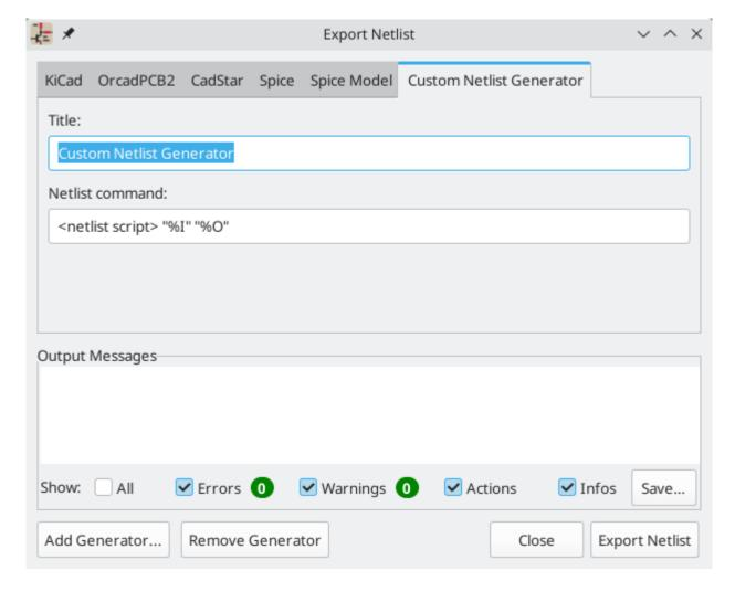
New generators require a name and a command. The name is shown in the tab label, and the command is run whenever the **Export Netlist** button is clicked.
