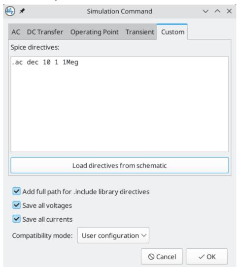
A custom analysis lets you write SPICE commands to set up the analysis. Press the **Load directives from schematic** button to copy any SPICE directives in schematic text into the custom analysis textbox.
