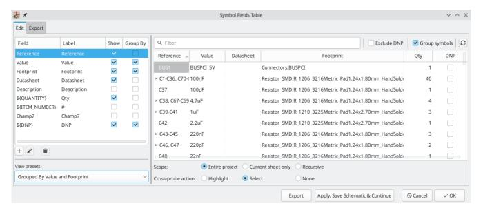
Fields with the **Show** box checked will be included as columns in the BOM, and fields with the **Group By** box checked are used to group components together. Components are grouped into the same line if all of their **Group By** fields are identical and the **Group symbols** box is checked. You can set an arbitrary column name for each field and reorder columns by dragging their headers.
