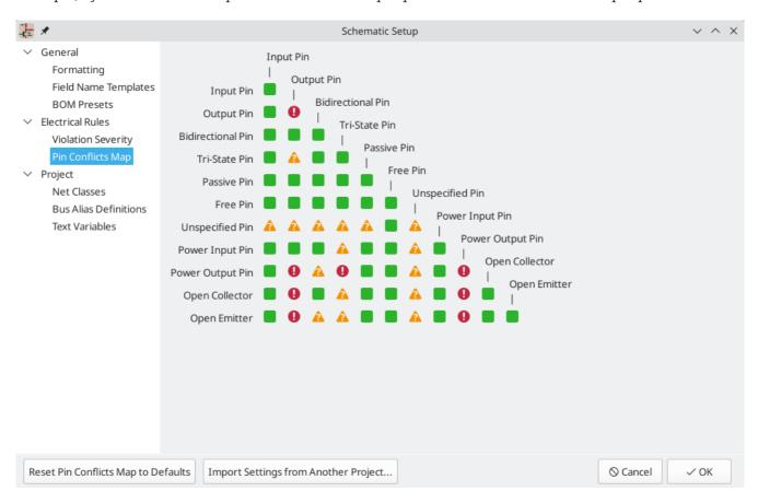
Rules can be changed by clicking on the desired square of the matrix, causing it to cycle through the choices: allowed, warning, error.
