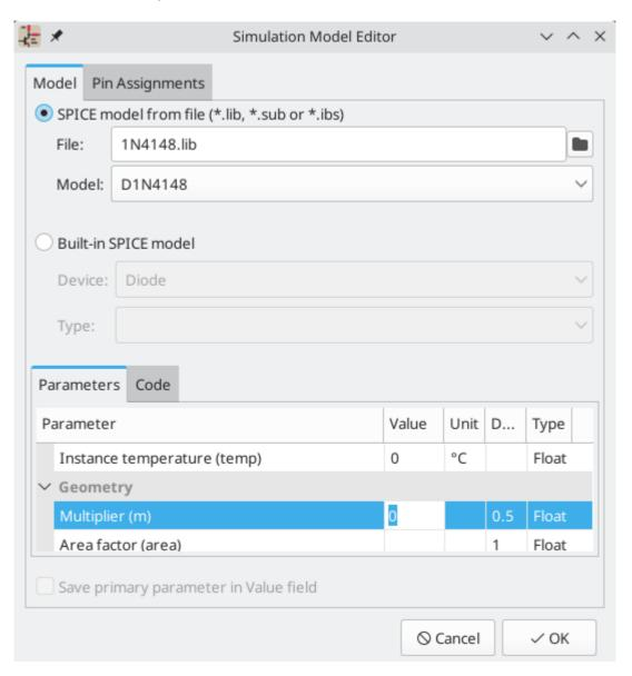
**File** is the path to the model file to use. Unencrypted model files are plain, human-readable text files and often have extensions such as .lib, .sub etc., although KiCad will accept a valid model with any extension.
