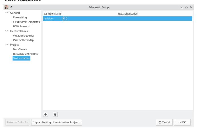
Text replacement variables can be created in the Text Variables section. These variables allow you to substitute the variable name for any text string. This substitution happens anywhere the variable name is used inside the variable replacement syntax of \${VARIABLENAME}.
