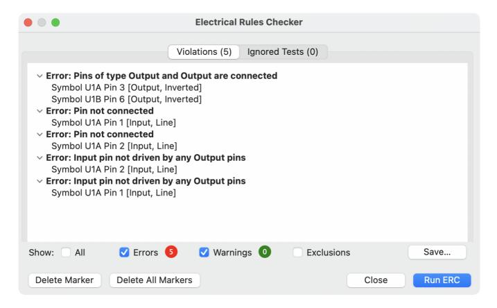
Any warnings or errors are reported in the **Violations** tab, and markers for each violation are placed in the schematic so that they point to the relevant part of the schematic. Warnings are indicated by yellow arrows, and errors have red arrows. Excluded violations are shown as green arrows.
