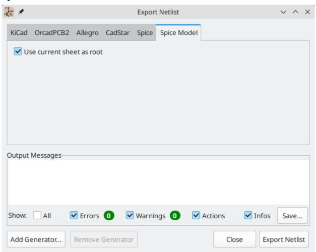
KiCad can also export a netlist of the schematic as a Spice subcircuit model, which can be included in a separate Spice simulation. Any hierarchical labels in the schematic are used as pins for the subcircuit model. Each pin in the model is annotated with a comment describing the pin's electrical direction:
