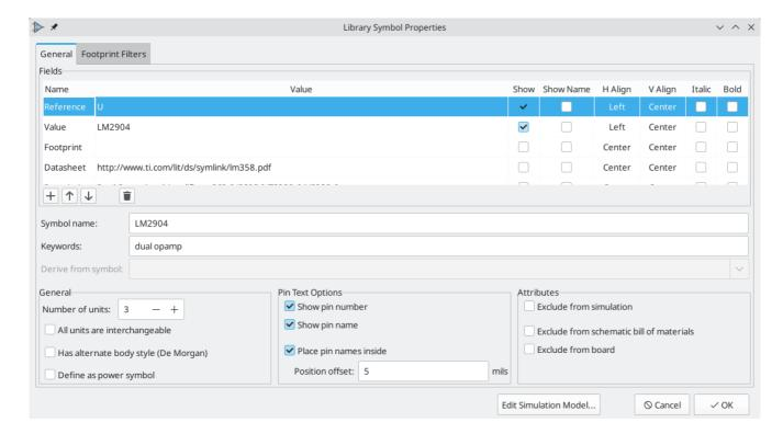
It is important to set the **number of units** and check **all units are interchangeable** and **has alternate body style**, as applicable, because these settings affect how pins and graphics are added to each symbol unit.
