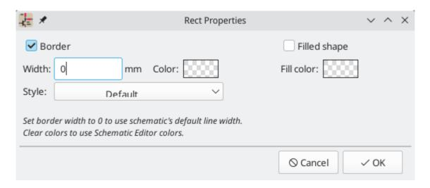
Setting a shape's line width to 0 uses the schematic default line width, which is configurable in Schematic Setup. Spacing for line dashes is also configurable there. Removing a line or fill color uses the color theme's graphics color, which is configurable in Preferences.
