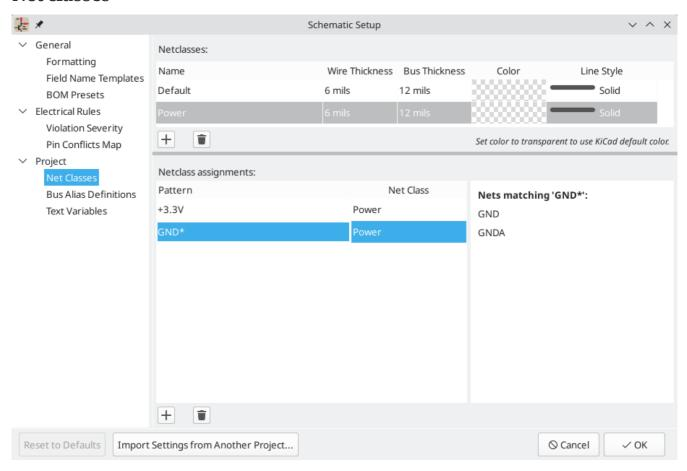
The **Net Classes** panel allows you to manage netclasses for the project and assign nets to netclasses with patterns. Managing netclasses in this panel is equivalent to managing them in the Board Setup dialog. Nets can also be assigned to netclasses in the schematic using graphical assignments with net class directives or net labels.
