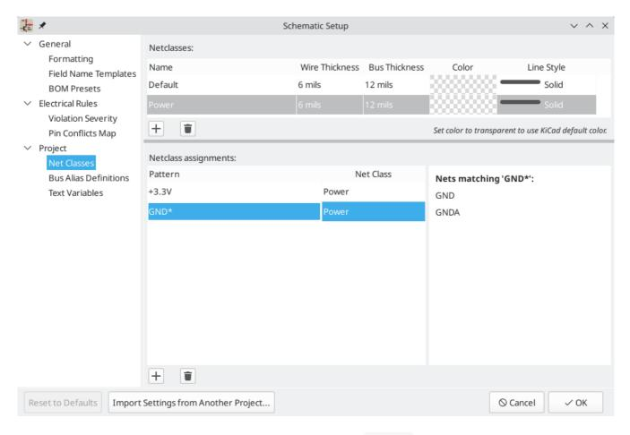
The top pane lists the netclasses that exist in the design. The Default netclass always exists, and you can add additional netclasses with the + button or remove the selected netclass with the = button.
