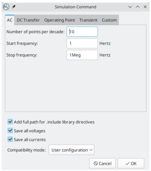
Calculates the small-signal AC behavior of the circuit in response to a stimulus. Performs a decade sweep of stimulus frequency.
