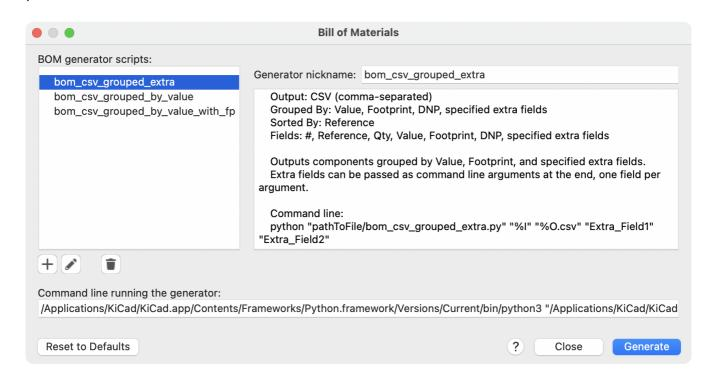
Several BOM generator scripts are included with KiCad, and users can also create their own. BOM generator scripts generally use Python or XSLT, but other tools can be used as long as you can specify a command line for KiCad to execute when running the generator.
