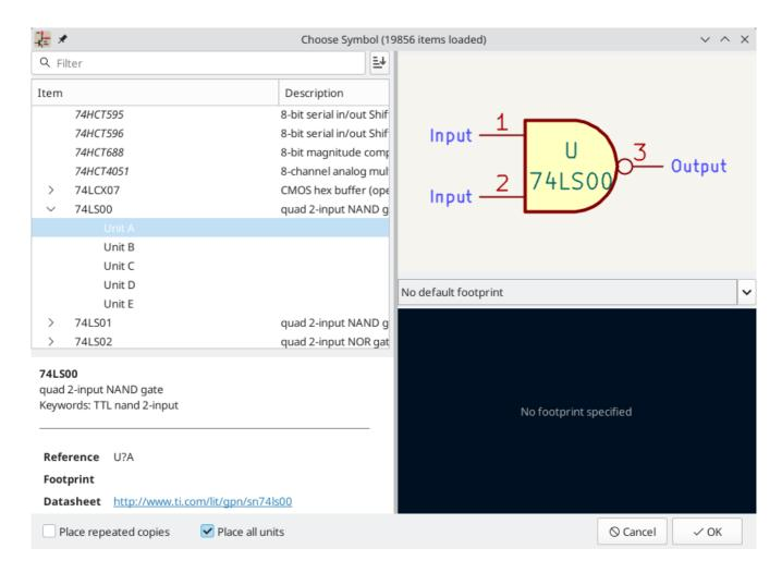
By default, only the symbol/library name and description columns are shown. Additional columns can be added by right-clicking the column header and selecting **Select Columns**.
