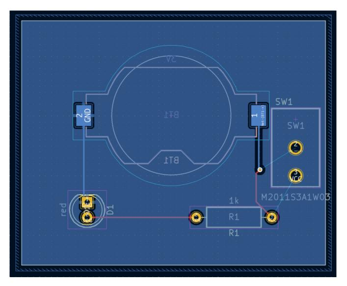
The ratsnest shows the new connections that need to be routed. Additionally, the connection between the battery and the resistor needs to be deleted.
