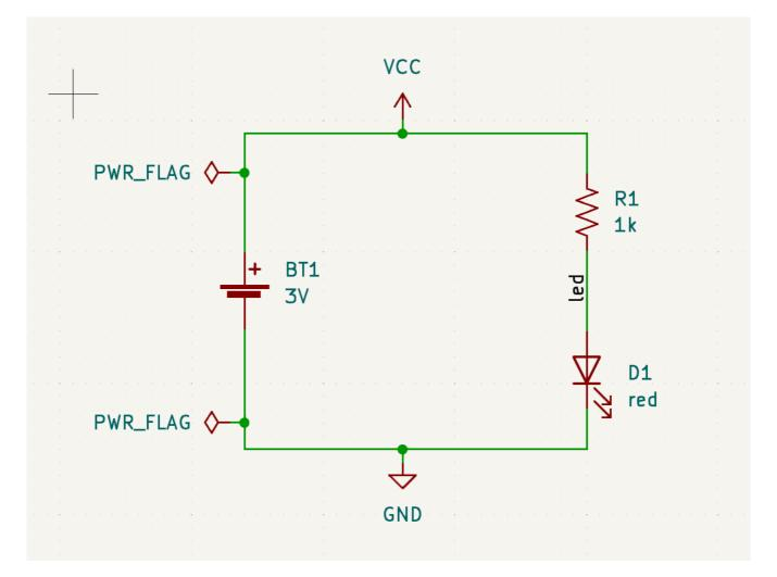
There is a special PWR\_FLAG symbol in the Power symbol library that is used to solve this problem by telling KiCad that the nets are actually driven. Add this symbol to the VCC and GND nets and re-run ERC. When ERC passes without any violations, the schematic is complete.
