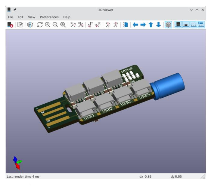
**NOTE** The 3D model for a component will only appear if the 3D model file exists and has been assigned to the footprint.
