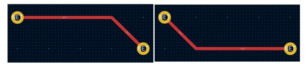
KiCad's router attempts to pick the best posture automatically based on a number of factors. In general, the router will attempt to minimize the number of corners in a route, and will avoid "bad" corners such as acute angles whenever possible. When routing from or to a pad, KiCad will choose the posture that lines up the route with the longest edge of the pad.
