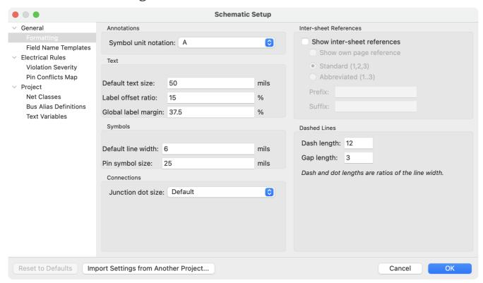
The formatting panel contains settings for the appearance of symbols, text, labels, graphics, and wires.
