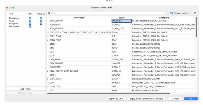
Cells are navigated with the arrow keys, or with Tab / Shift + Tab to move right / left and Enter / Shift + Tab to move down / up, respectively.
