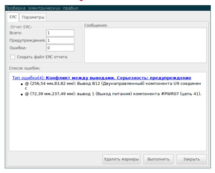
Any warnings or errors are reported in the **Violations** tab, and markers for each violation are placed in the schematic so that they point to the relevant part of the schematic. Warnings are indicated by yellow arrows, and errors have red arrows. Excluded violations are shown as green arrows.
