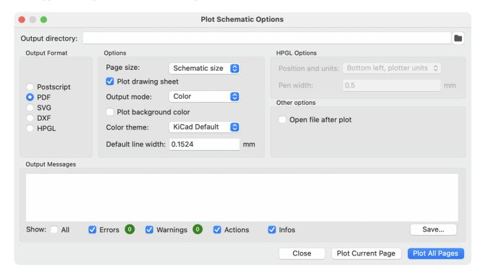
The **Output Messages** pane displays messages about the generated files. Different kinds of messages can be shown or hidden using the checkboxes, and the messages can be saved to a file using the **Save...** button.
