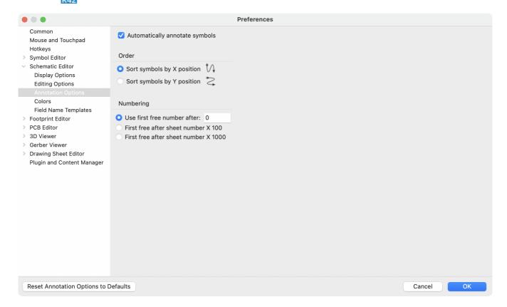
When multiple symbols are added simultaneously, they are annotated according to the **Order** setting, sorted by either X or Y position.
