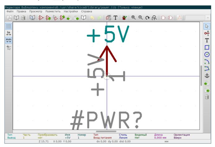
Power symbols consist of a pin of type "Power input" that is marked invisible. They must also have the **Define as power symbol** property checked. **Invisible power input pins** have a special property of making implicit global connections based on the pin name.
