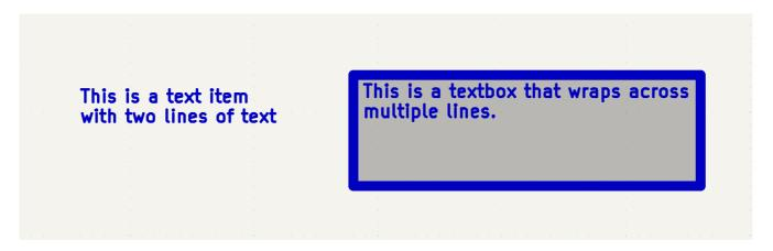
Both kinds of text item support multiline text and basic formatting features, but text boxes wrap text to fit in the outline and have additional formatting options. All text has adjustable fonts, color, size, bold and italic emphasis, left and right alignment, and vertical and horizontal orientation. Text boxes additionally support horizontal centering, vertical alignment options, and colored borders and fill.
