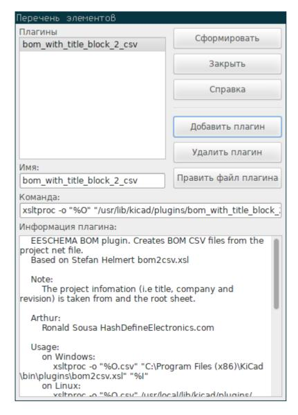
Additional scripts can be added to the list of BOM generator scripts by clicking the + button. Scripts can be removed by clicking the = button. The  $\nearrow$  button opens the selected script in a text editor.
