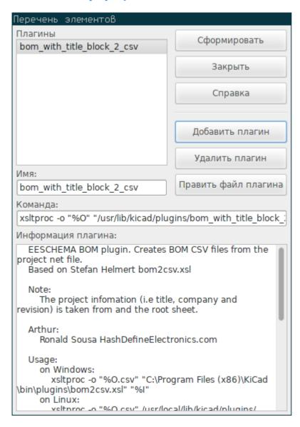
The BOM tool uses an external script to process the design information into the desired output format. Several BOM generator scripts are included with KiCad, and users can also create their own. BOM generator scripts generally use Python or XSLT, but other tools can be used as long as you can specify a command line for KiCad to execute when running the generator.
