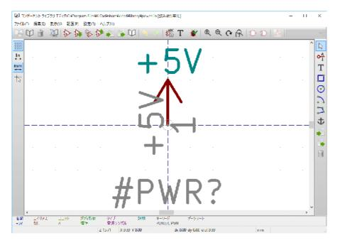
Power symbols consist of a pin of type "Power input" that is marked invisible. They must also have the **Define as power symbol** property checked. Invisible power input pins have a special property of making implicit global connections based on the pin name.
