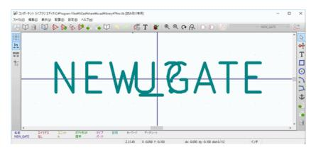
The blue cross in the center is the symbol anchor, which specifies the symbol origin i.e. the coordinates (0, 0). The anchor can be repositioned by selecting the 400 icon and clicking on the new desired anchor position.
