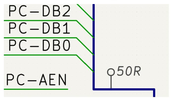
Net class directives are added with the  $\mathbf{Q}\mathbf{A}$  button in the right toolbar. They behave like labels, except that they cannot be used to name a net. The attached net is assigned a netclass according to the value of the directive's Net Class field. The Net Class field presents a dropdown list of all the net classes in the design.
