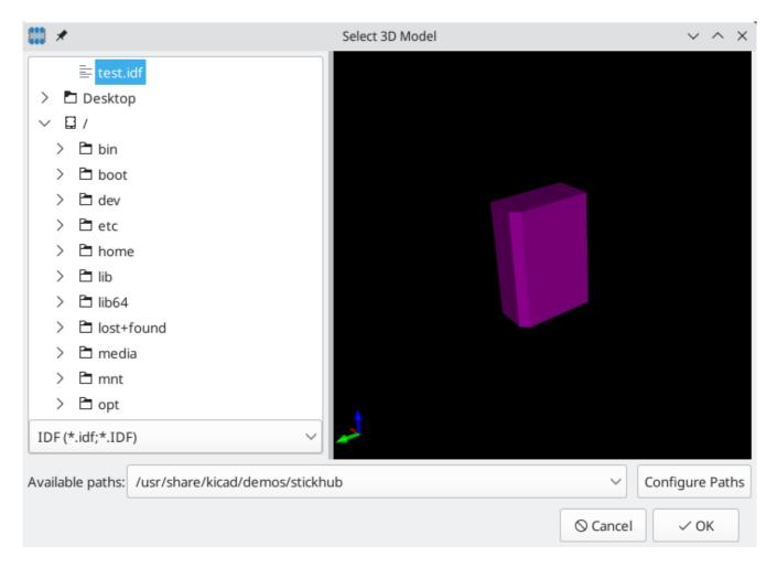
Once the desired component outline file is selected, enter any necessary values for the offset and rotation. The offsets must be specified using the IDF board output units (mm or mils) and in the IDF coordinate system, which is a right-hand coordinate system with +Z pointing towards the viewer, +X to the viewer's right, and +Y towards the upper edge of the screen. The rotation must be in degrees; positive rotation is a counter-clockwise rotation as described in the IDFv3 specification.
