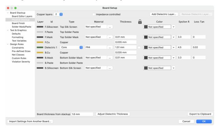
Set the number of copper layers in the upper left corner and then enter the physical parameters of the stackup if desired. These parameters may be left at their default values, but note that the board thickness value will be used when exporting a 3D model of the board. If you plan to use this feature, it is a good idea to ensure that the stackup thickness is correct.
