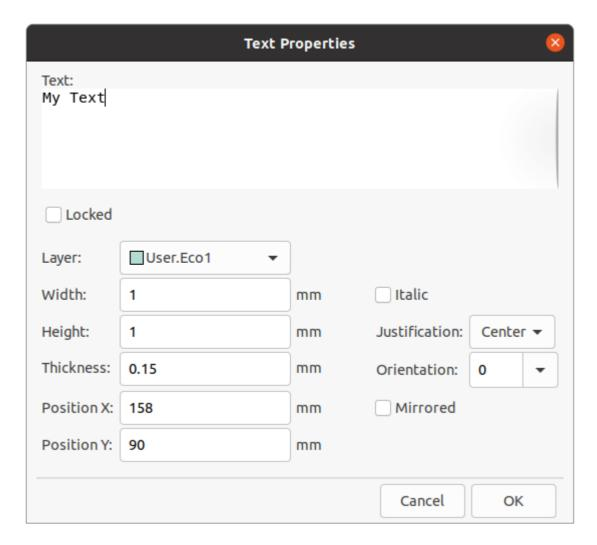
Text may be placed on any layer, but note that text on copper layers cannot be associated with a net and cannot form connections to tracks or pads. Copper zones will fill around the rectangular bounding box of text objects.
