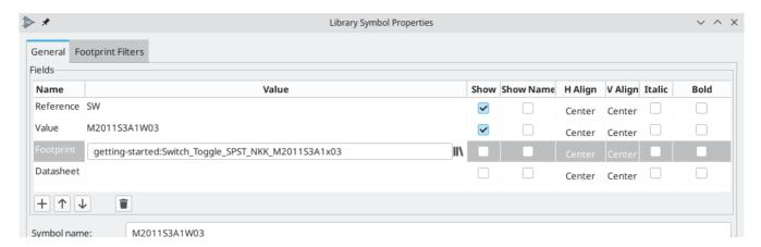
Symbols can specify a preselected footprint. Footprints do not need to be manually assigned to such symbols, because a footprint was chosen when the symbol was created. Users can override the preselected footprint during the footprint assignment process as normal. Defining a default footprint is a good idea for
