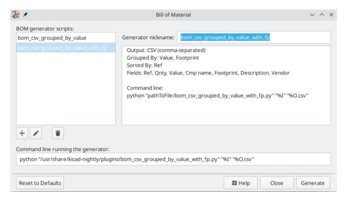
KiCad 7.0 uses Python scripts to generate BOMs. Three BOM scripts are included, and users can also create their own scripts to generate BOMs in whatever format is desired.
