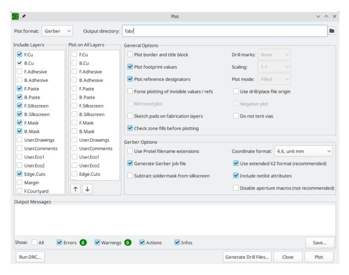
Click **Plot** to generate the Gerber files. Also click **Generate Drill Files...** and then **Generate Drill File** to create files specifying the location of all holes that will be drilled in the board. Finally, close the Plot dialog. The design is finished.
