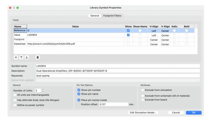
It is important to set the **number of units** and check **all units are interchangeable** and **has alternate body style**, as applicable, because these settings affect how pins and graphics are added to each symbol unit.
