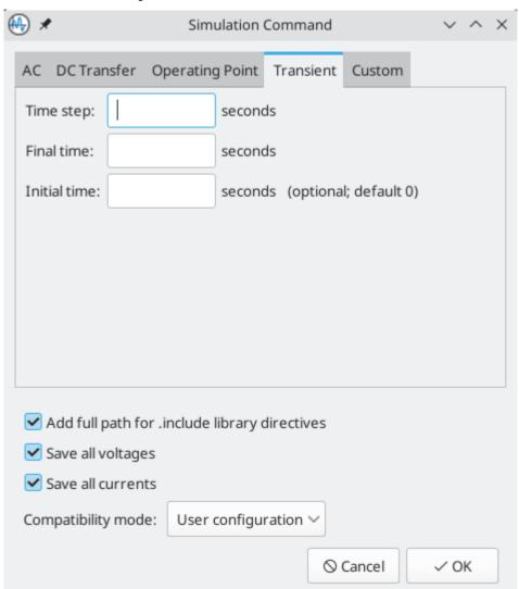
Calculates the time-varying behavior of the circuit.
