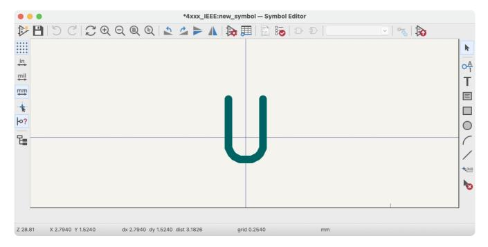
The blue cross in the center is the symbol anchor, which specifies the symbol origin i.e. the coordinates (0, 0). The anchor can be repositioned by selecting the \*@@ icon and clicking on the new desired anchor position.
