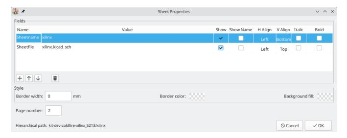
The **sheet name** must be unique, as it is used in the full net name for any nets in the subsheet. For example, a net with the local label net1 in the sheet sheet1 would have a full net name of /sheet1/net1. The sheet name is also used to refer to the sheet in various places in the GUI, including the title block and the hierarchy navigator.
