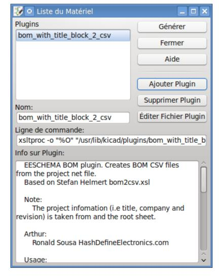
Additional scripts can be added to the list of BOM generator scripts by clicking the + button. Scripts can be removed by clicking the = button. The  $\nearrow$  button opens the selected script in a text editor.
