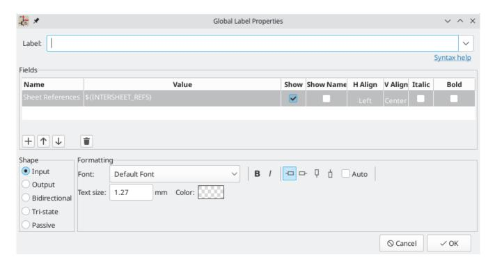
The **Label** field sets the label's text, which determines the net that the label assigns to its attached wire. Label text supports markup for overbars, subscripts, etc., as well as variable substitution. Use the **Syntax help** link in the dialog for a summary.
