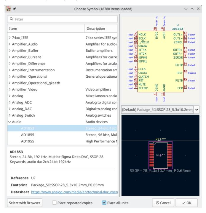
Symbols can have footprint filters that specify which footprints are appropriate to use with that symbol. If footprint filters are defined for the selected symbol, all footprints that match the footprint filters will appear as options in the footprint dropdown. The selected footprint will be displayed in the preview canvas and will be assigned to the symbol when the symbol is added to the schematic.
