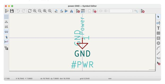
Power symbols consist of a pin of type "Power input" that is marked invisible. They must also have the **Define as power symbol** property checked. **Invisible power input pins** have a special property of making implicit global connections based on the pin name.
