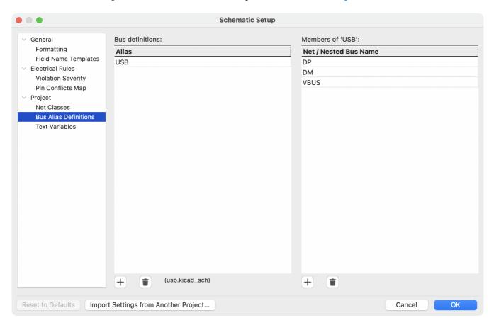
An alias may be named any valid signal name. Using the dialog, you can add signals or vector buses to the alias. As a shortcut, you can type or paste in a list of signals and/or buses separated by spaces, and they will all be added to the alias definition. In this example, we define an alias called USB with members DP, DM, and VBUS.
