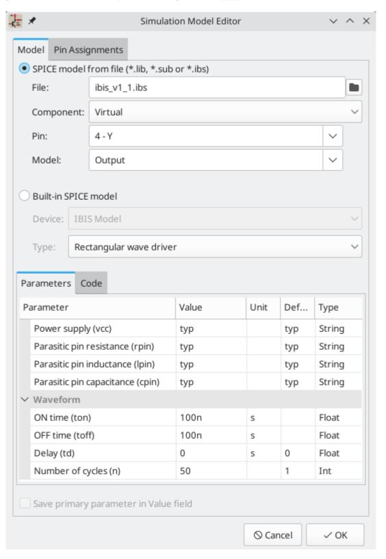
**File** is the path to the model file to use. The path can be absolute or relative to the project folder. The path can also be relative to the value of SPICE\_LIB\_DIR if you have defined that path variable. The library filename is saved in the symbol's Sim.Library field. If an IBIS model file is loaded, the remaining fields in the dialog will relate to the IBIS model.
