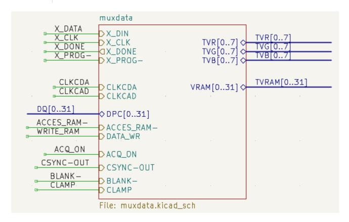
For every hierarchical label in the subsheet, import the corresponding hierarchical pin into the sheet symbol by clicking the button in the right toolbar, then clicking on the sheet symbol. A sheet pin for the first
