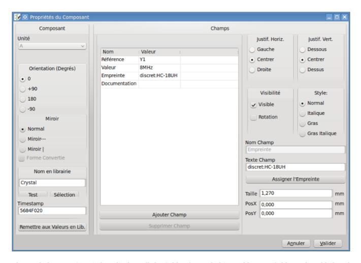
The Symbol Properties window displays all the fields of a symbol in a table. New fields can be added, and existing fields can be deleted, edited, reordered, moved, or resized.
