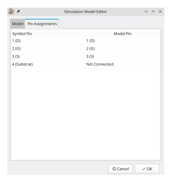
The left column displays the name and number of each symbol pin. For each symbol pin, you can select the corresponding pin from the simulation model in the dropdown in the right column.
