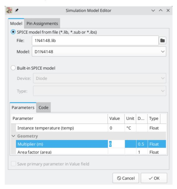
**File** is the path to the model file to use. The path can be absolute or relative to the project folder. The path can also be relative to the value of SPICE\_LIB\_DIR if you have defined that path variable. The library filename is saved in the symbol's Sim.Library field.
