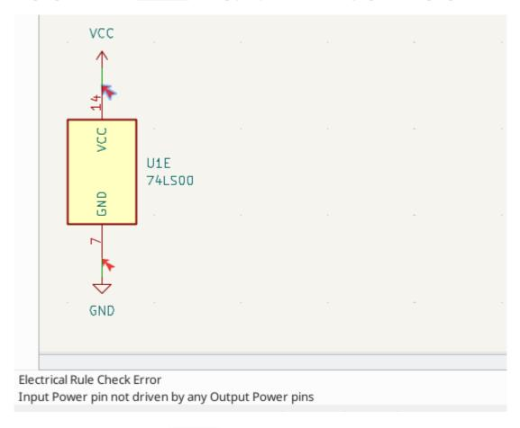
Ground nets often need a PWR\_FLAG as well, because voltage regulators have outputs declared as power outputs, but their ground pins are typically marked as power inputs. Therefore grounds can appear unconnected to a source unless a PWR\_FLAG symbol is used.
