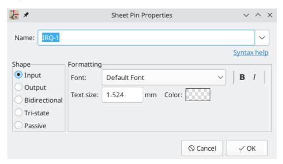
The sheet pin's **name** can be edited in the textbox or by selecting from the dropdown list of hierarchical labels in the subsheet. A sheet pin's name has to match the corresponding hierarchical label in the subsheet, so if a pin name is changed the label must change as well.
