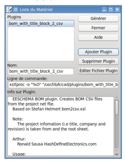
The BOM tool uses an external script to process the design information into the desired output format. Several BOM generator scripts are included with KiCad, and users can also create their own. BOM generator scripts generally use Python or XSLT, but other tools can be used as long as you can specify a command line for KiCad to execute when running the generator.
