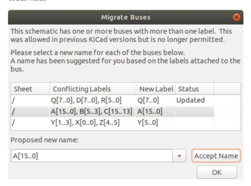
For each set of bus wires that has more than one label, you must choose the label to keep. The drop-down name box lets you choose between the labels that exist in the design, or you can choose a different name by manually entering it into the new name field.
