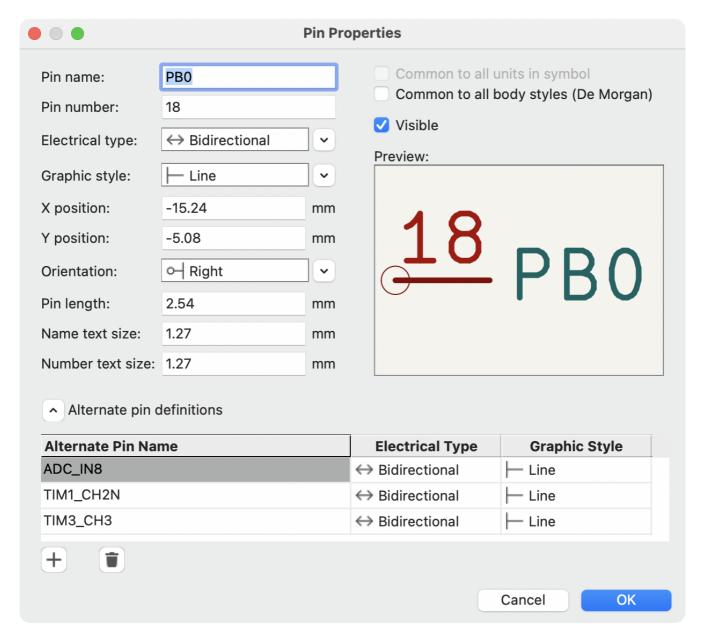
Alternate pin definitions are selected in the Schematic Editor once the symbol has been placed in the schematic. The alternate pin is assigned in the Alternate Pin Assignments tab of the Symbol Properties dialog. Alternate definitions are selectable in the dropdown in the Alternate Assignment column.
