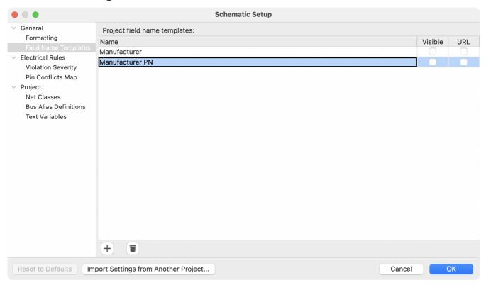
Field name templates are empty symbol fields that are automatically added to all symbols in the schematic. These can be useful when every symbol in the schematic needs additional fields beyond the fields that are defined in the library symbols, for example a field for the manufacturer's part number.
