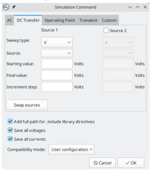
Calculates the DC behavior of the circuit while sweeping one or two sources (voltage or current), resistors, or the simulation temperature.
