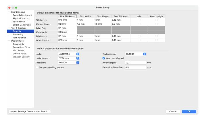
Line thickness, text size, and text appearance can be configured for the six different categories of layers shown in the dialog. Additionally, the properties for dimension objects can be configured for all layers. For more details about dimension properties, see the Dimensions section below.
