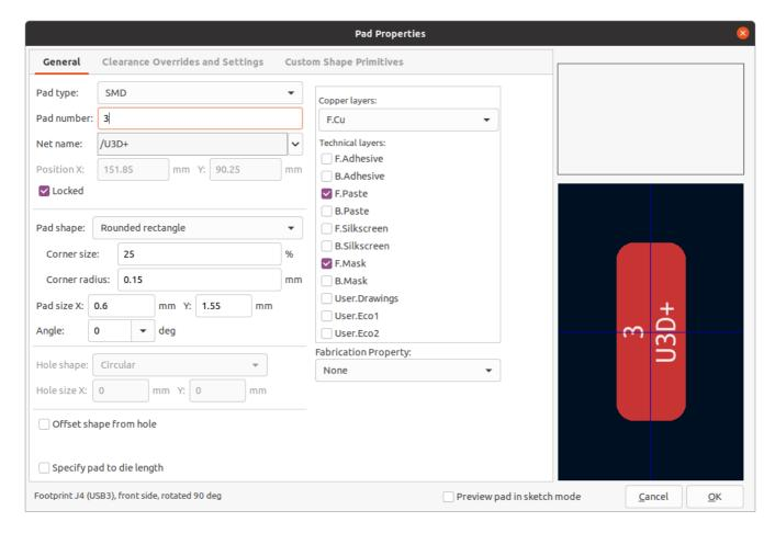
The General tab of the pad properties dialog shows the physical properties of the pad, including its geometry, shape, and layer settings.
