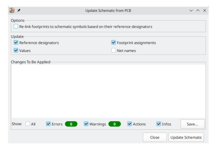
The tool syncs changes in reference designators, values, footprint assignments, and net names from the board to the schematic. Each type of change can be individually enabled or disabled.
