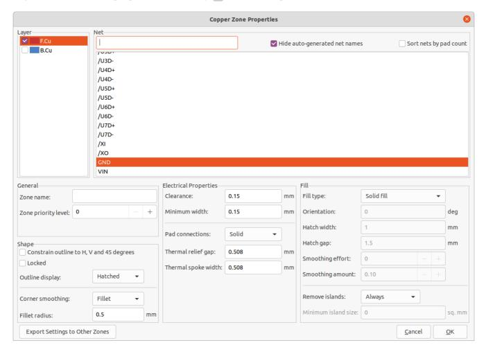
**Layer:** A single zone object can create filled copper on one or more copper layers. Check the box next to each copper layer that this zone outline should fill on. The copper on each layer will be filled independently, but all layers will share the same net.
