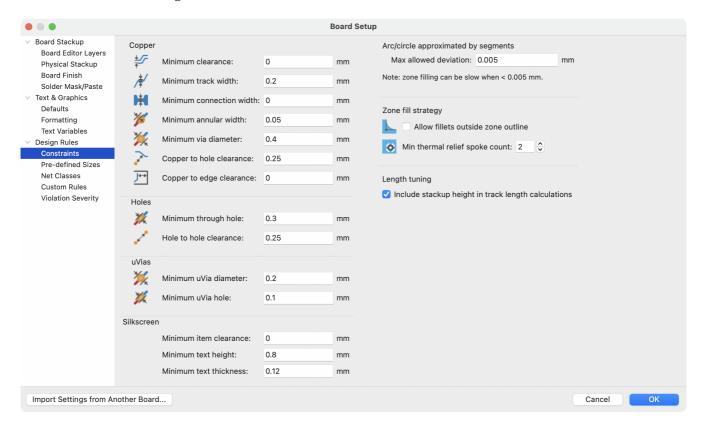
In addition to setting minimum clearances, a number of features can be configured here:
