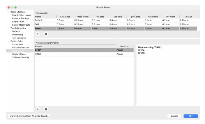
The upper portion of the Net Classes section contains a table showing the net classes in the design and the design rules that apply to each net class. Every class has values for copper clearance, track width, via sizes,
