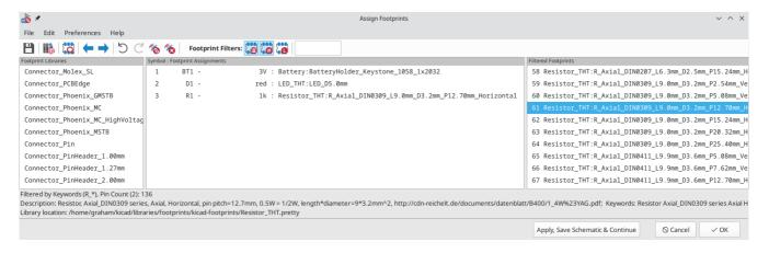
Many footprints are included with KiCad, so the footprint assignment tool offers several ways to filter out footprints that aren't relevant to the symbol in question.
