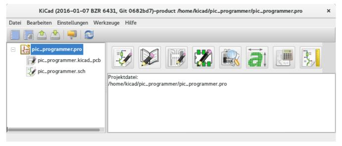
The KiCad project manager window is composed of a tree view on the left showing the files associated with the open project, and a launcher on the right containing shortcuts to the various editors and tools.
