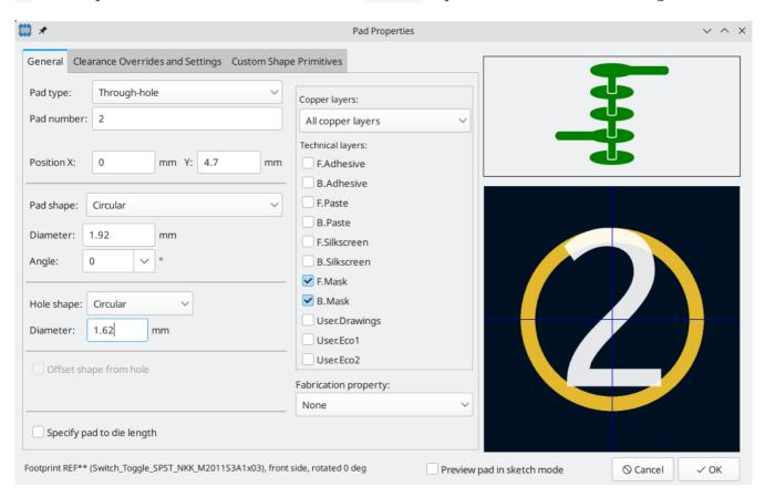
Now use the **Add a pad** tool again to place the other pad at (0, 9.4 mm). Notice that the pad number is automatically incremented and the properties including pad size and hole size are copied from the previous pad.
