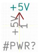
Power symbols consist of a pin of type "Power input" that is marked invisible. They must also have the **Define as power symbol** property checked. Invisible power input pins have a special property of making implicit global connections based on the pin name.
