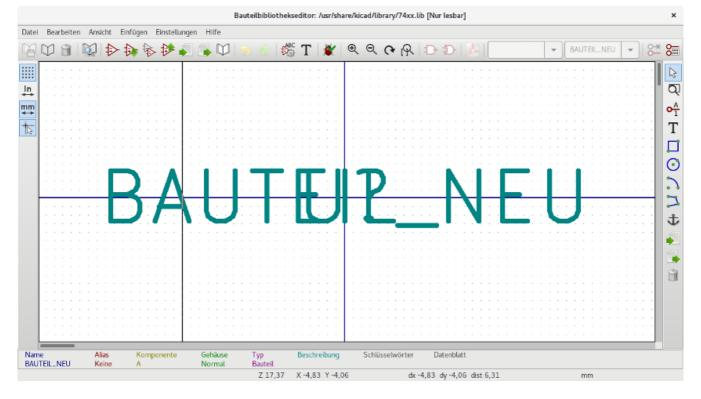
The blue cross in the center is the symbol anchor, which specifies the symbol origin i.e. the coordinates (0, 0). The anchor can be repositioned by selecting the **\***<sup>[00]</sup> icon and clicking on the new desired anchor position.
