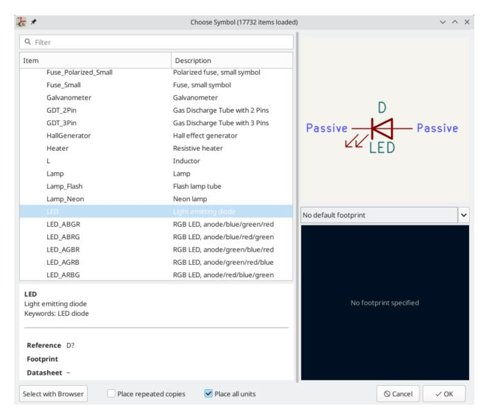
Next, add a current-limiting resistor. Go back to the symbol chooser, but this time try searching for a resistor by entering R in the filter box at the top. Again, it is found in the Device library. The R device is an IEC-style rectangular resistor symbol. An R\_US symbol is also available for users who prefer the ANSI-style zigzag symbol. Select a resistor symbol and add it to the schematic.
