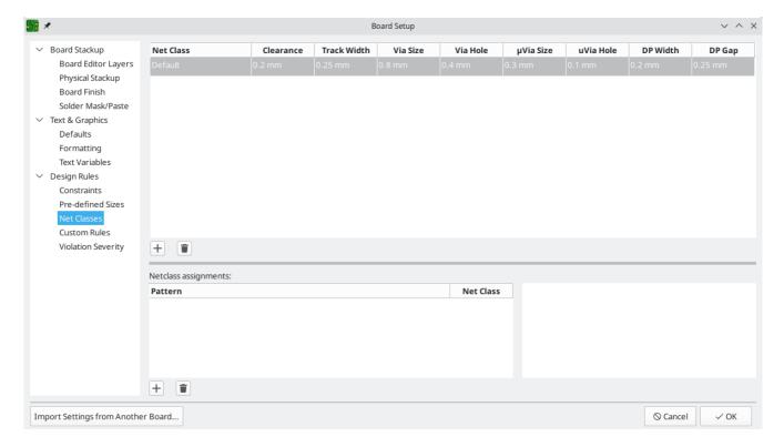
Track width and spacing can be managed manually by the designer during layout, but net classes are recommended because they provide an automatic way to manage and check design rules.
