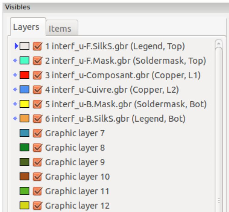
The Layers Manager controls and displays visibility of all layers. An arrow indicates the active layer, and each layer can be shown or hidden with the checkboxes.
